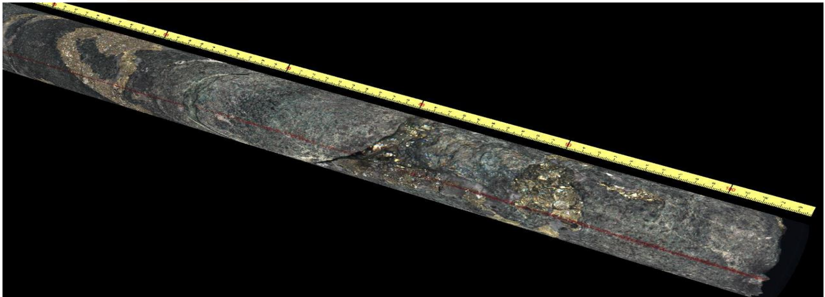
Drillcore intercept from ALCA002 (227.69m to 228.19m) showing chalcopyrite/pyrite mineralisation within a chlorite altered quartz-tourmaline breccia zone in a wider zone of weakly potassic altered monzonite.
