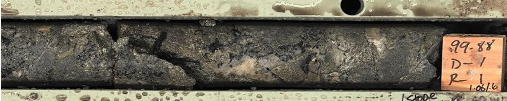
Hole ALCA001 (99.8m) showing quartz-tourmaline-pyrite chalcopyrite breccia with estimated chalcopyrite abundance of 5-10% and pyrite abundance of 5-10%.
