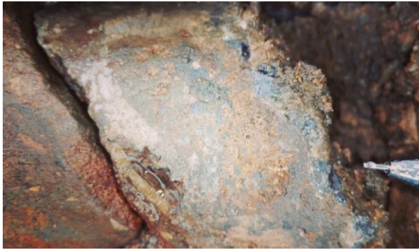
Figure 7: LEFT Close up core photo at 96m down hole depth in RDDH-020. Pictured is an example of a vein with coarse galena and Fe-oxides. The sample corresponding to this core photo grades 2.72% Zn, 45.1g/t Ag and 3.61% Pb .
