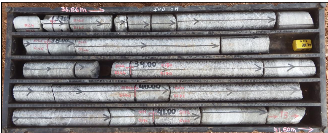
Figure 4: Graphitic gneiss (~ 7% TGC) between 36.86–41.5 m downhole in IVD019. Mineralisation zone 2.
