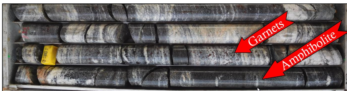
Figure 7: Footwall amphibolite, with garnetiferous zone near top contact in IVD008.
