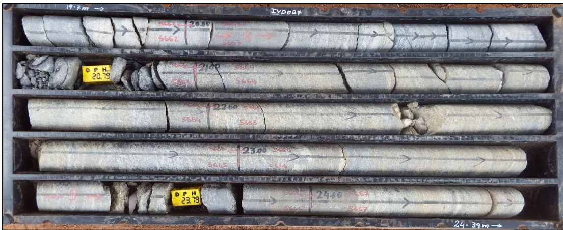
Figure 3: Graphitic gneiss (~ 7% TGC) between 19.7–24.4 m downhole in IVD027. Mineralisation zone 15.
