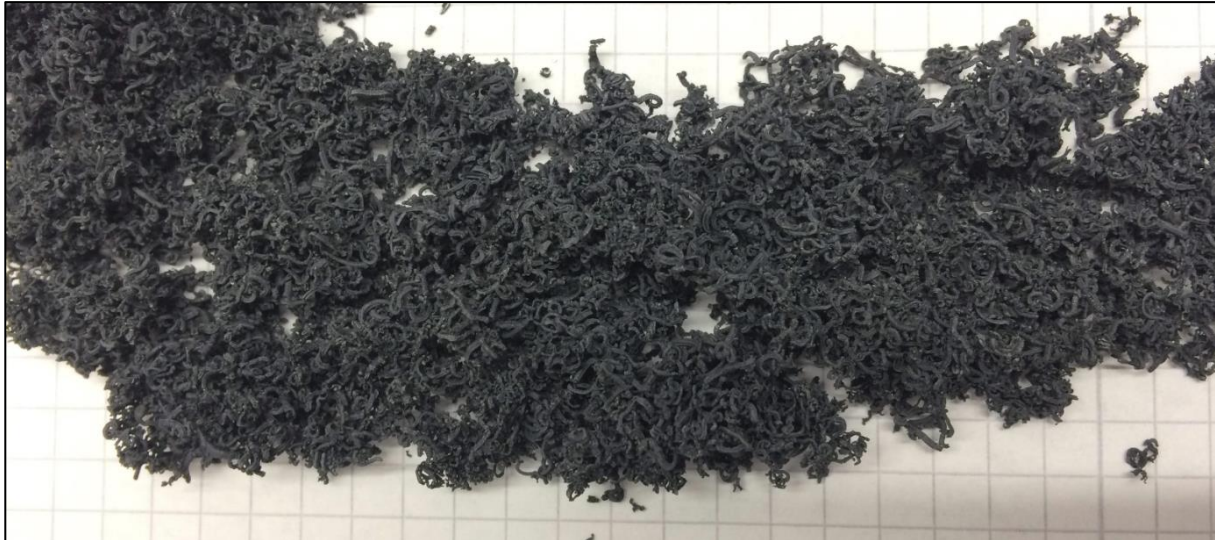
Figure 24: Ancuabe +50 mesh concentrate converted to expandable graphite and exfoliated
