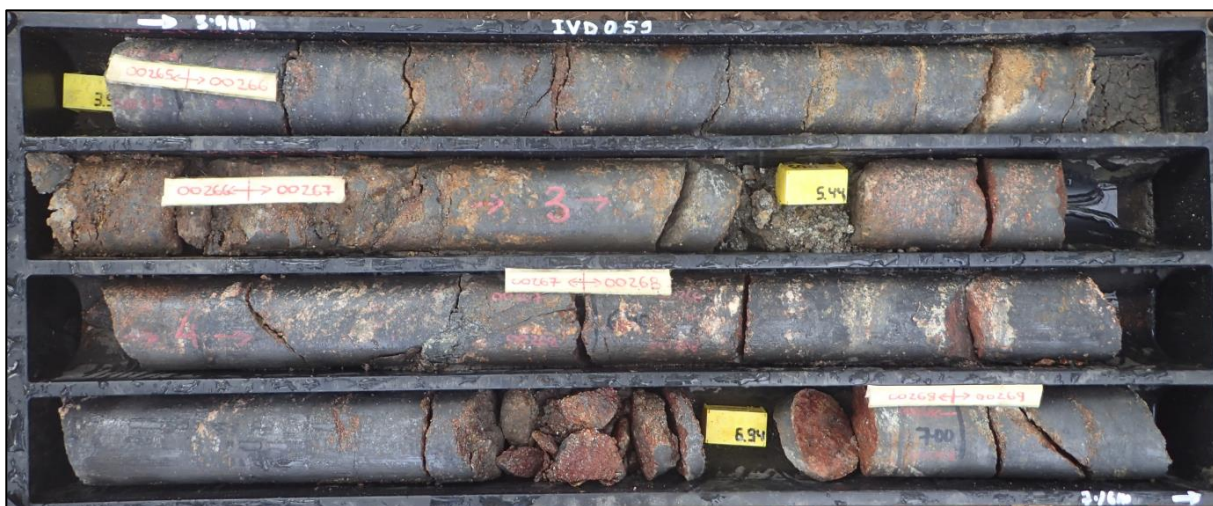
Figure 3: Oxidised graphite gneiss between 3.94 m and 7.16 m in IVD059 (~ 10% TGC)
