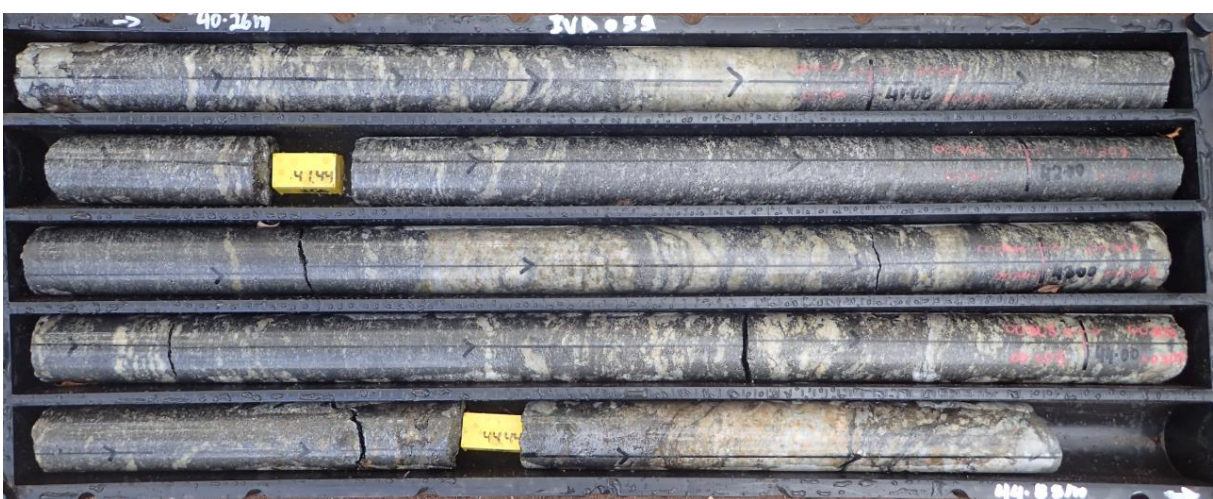
Figure 4: Fresh graphitic gneiss from 40.26 m to 44.85 m in IVD059 (~ 9% TGC)
