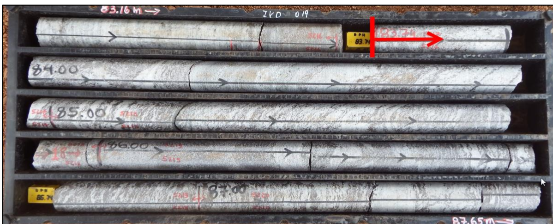
Figure 5: Graphitic gneiss (~ 6% TGC) between 83.74–87.65 m downhole in IVD019. Mineralisation zone 1.
