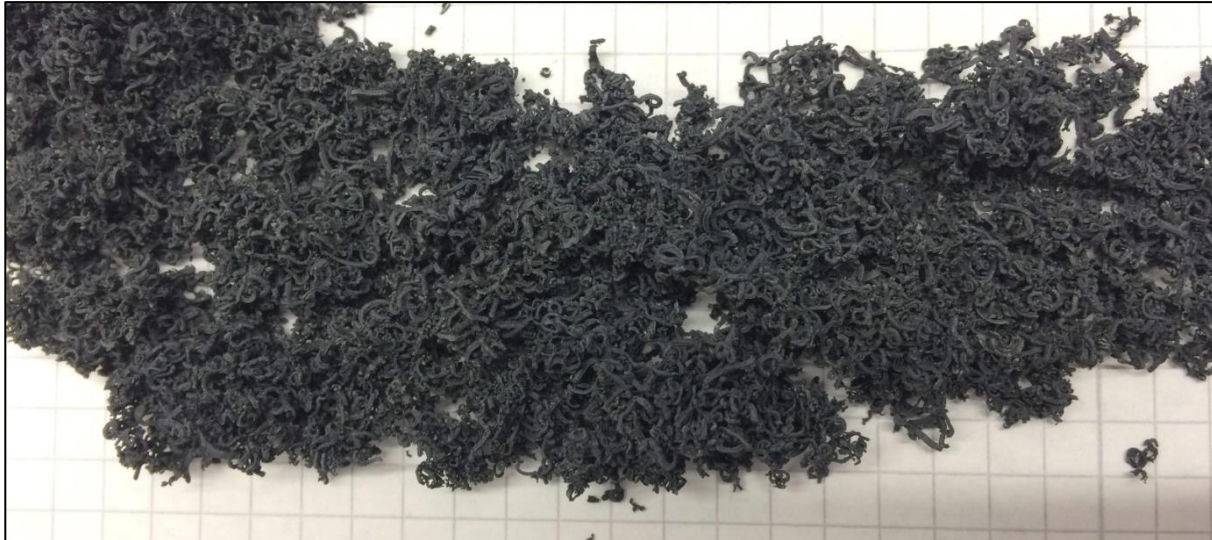
Figure 22: Ancuabe +50 mesh concentrate converted to expandable graphite and exfoliated to >320 mL/g
