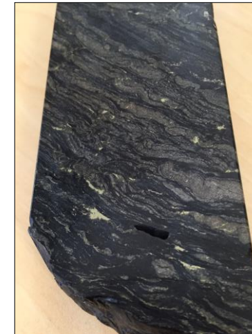
Disseminated chalcopyrite in carbonaceous shale EPT 2282 ~259.2m downhole (1.0% Cu)
