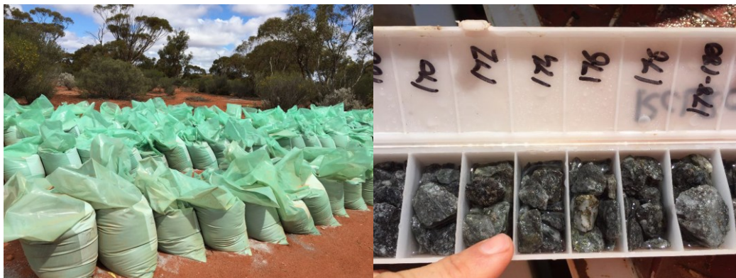
Photos – RC sample bags (left), sulphidic altered gneiss in RC chips RCLR0208 (right)
