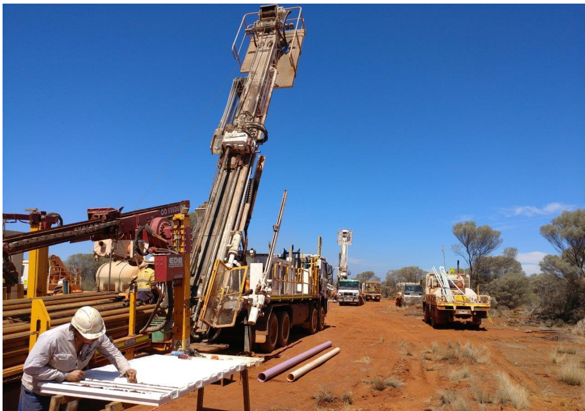
Figure 4. Diamond and RC drill rigs in operation at Mt Venn
