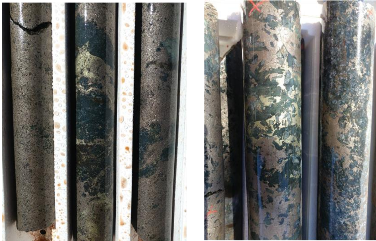
Figure 1. Diamond drill hole 17MVDD001 (LHS) - Massive pyrrhotite with chalcopyrite at 105m downhole Diamond tail 17MVRCD008 (RHS) – Semi-massive and stringer pyrrhotite with chalcopyrite at 113m downhole
