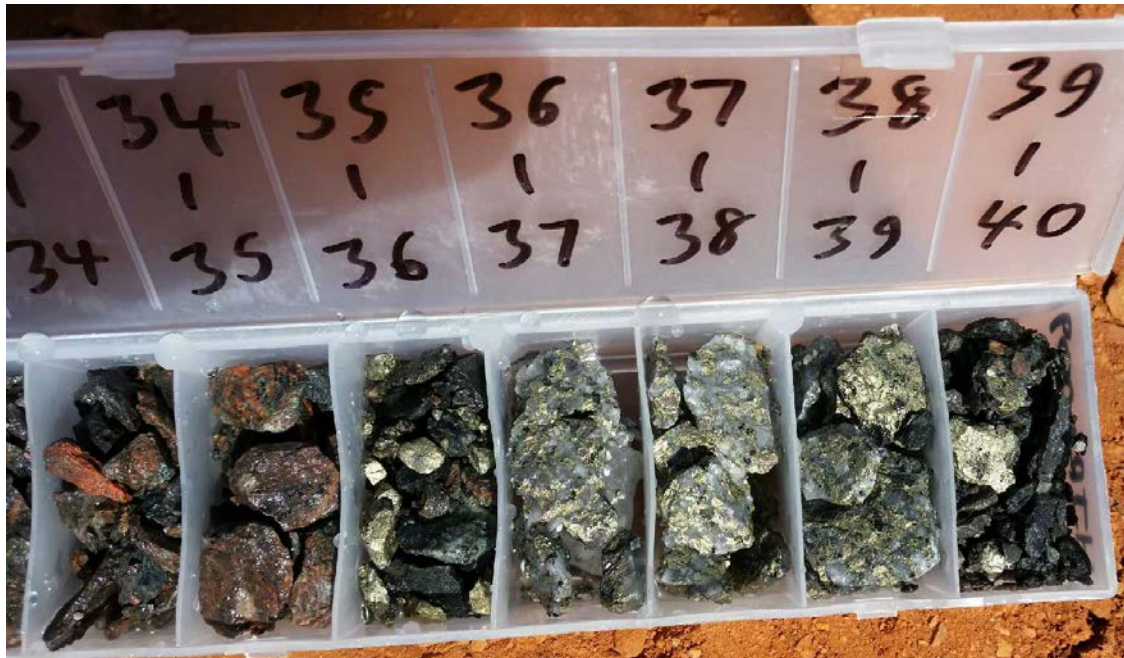
HJRC 009 33 – 40 metres with visible pyrite, pyrrhotite and chalcopyrite
