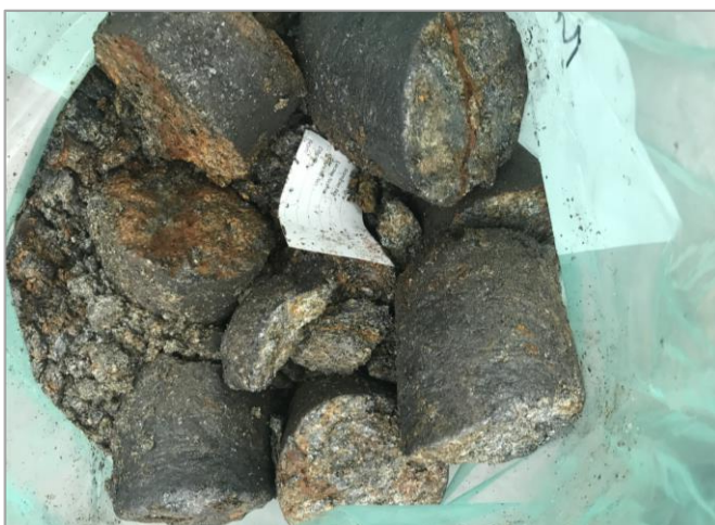
Figure 3a (LHS): PQ drill core sample from Malingunde ready for the scrubbing test-work program.
