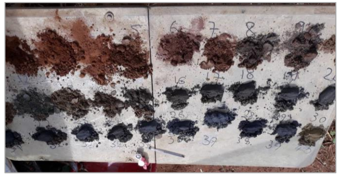
Figure 1b (RHS): High-grade graphitic-saprolite (8-29m downhole) in samples from Malingunde South Extension.
