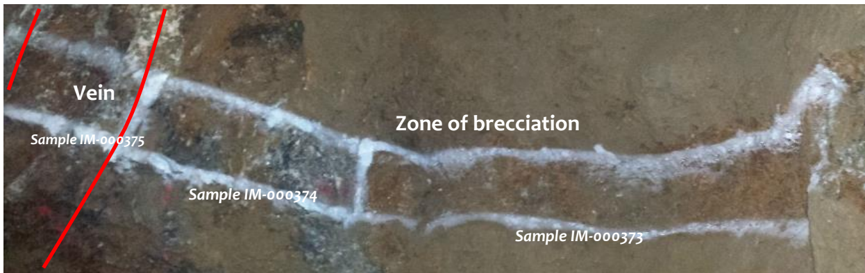
Figure 2 ABOVE: Underground photo of gallery 1, channel 6, which averages 9.7% Zn, 29.4g/t Ag, 2.72% Pb over 2.05m.
