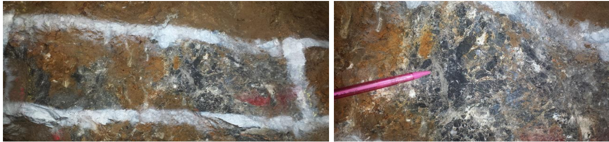
Figure 3 ABOVE LEFT: Underground photo showing channel sample IM-000374. Mineralisation at this location is associated with a broad breccia zone. ABOVE RIGHT: Underground photo showing detail of channel sample IM-000374. The breccia clasts are sub-rounded to angular which is indicative of sustained and repeated brecciation (or rock breaking events). IM-000374 grades 18.23% Zn, 25.8g/t Ag, 0.29% Pb.
