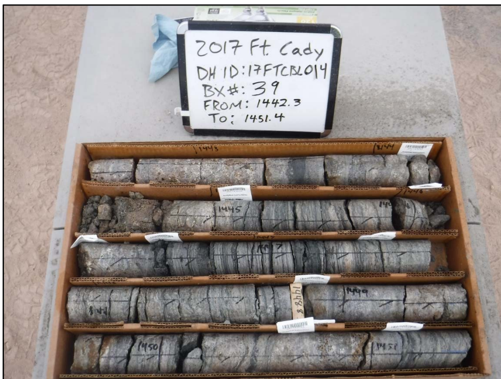
Figure 11. Core photo, 17FTCBL-0014, Note the variability of the core, including finely banded clay, and more competent evaporitic (mostly anhydrite, the lightest coloured material) sections. Depth measurements are in feet.
