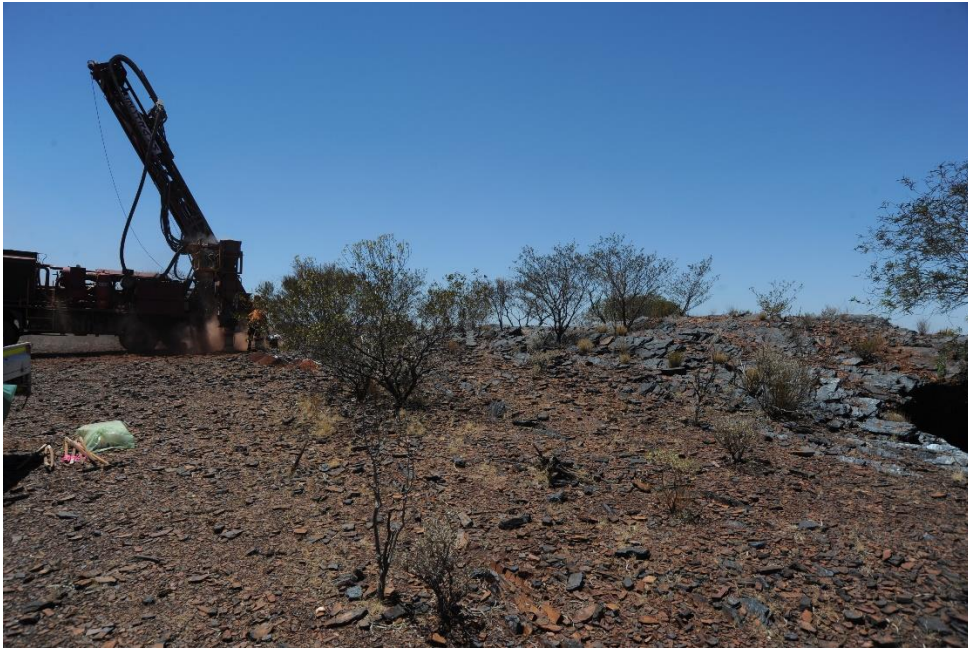
Figure 2: Drilling into outcropping manganese-mineralised sediments at the Pools prospect.
