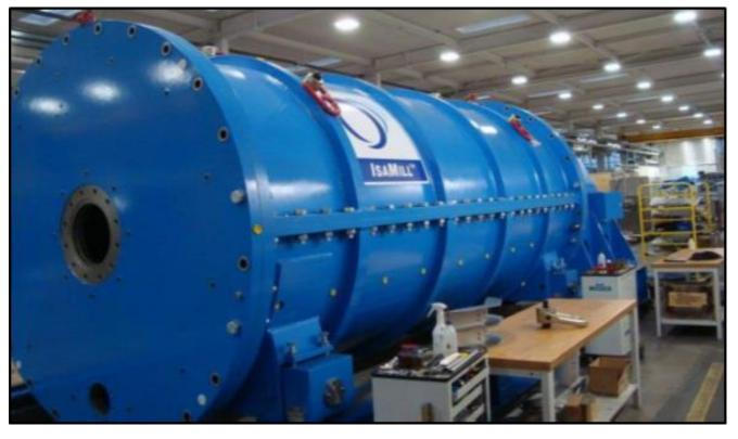
Figure 6: Woodlawn's IsaMill M10000 shell – original critical path item that is ahead of the forecast fabrication schedule.
