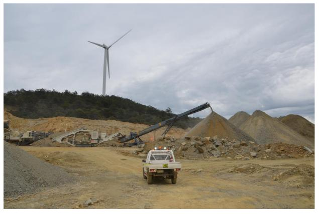
Figure 4: One of two on-site crushers producing final pavement material.
