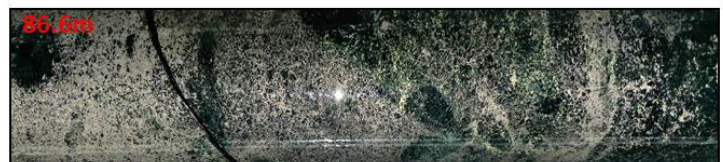
17MVDD002 (83.6-87.1m) – Stringer and heavily disseminated chalcopyrite at the margins of massive pyrrhotite
