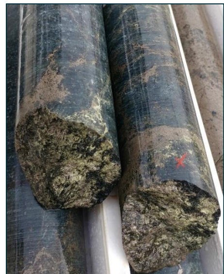
17MVDD002 – Stringer chalcopyrite and pyrrhotite mineralisation (109m)
