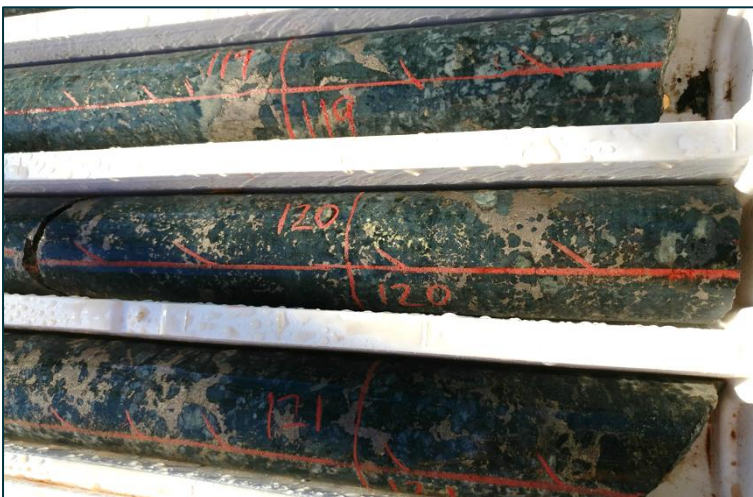
Top: 17MVDD003 (97.5m) – Band of massive pyrrhotite and chalcopyrite
