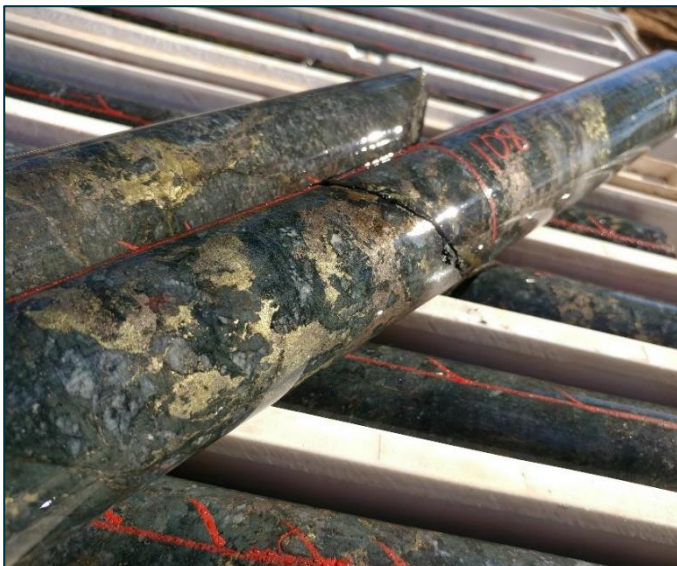
17MVDD003 – Western copper zone with interstitial chalcopyrite and pyrrhotite within very coarse-grained gabbro (108m)
