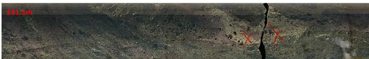
17MVDD003 (139.2-143.5m) –Semi-massive, blebby and stringer chalcopyrite and pyrrhotite
