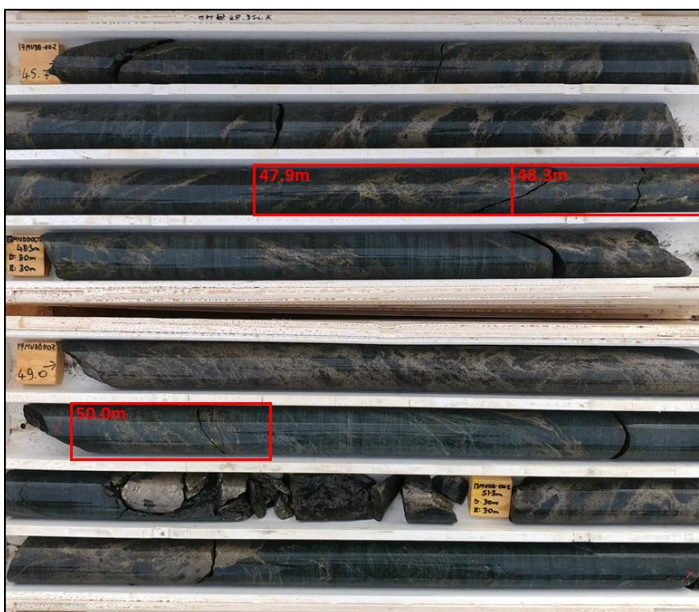
17MVDD002 (45.7m-52.5m) – Semi-massive and stringer pyrrhotite and chalcopyrite in meta-dolerite
