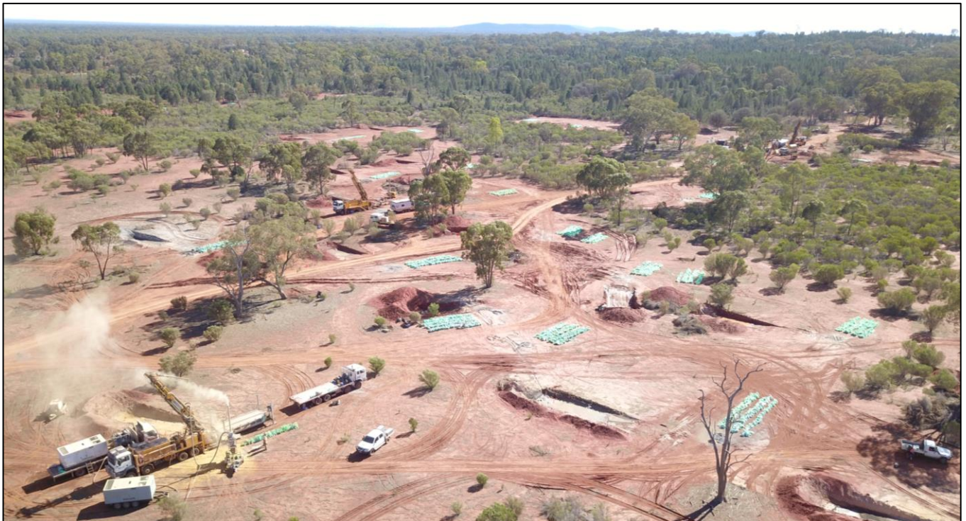
Figure 1: Southern Nights drill area – 1 x RC rig (nearest), 2 x diamond rigs
