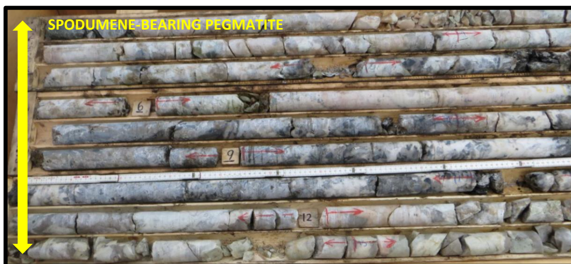
Figure 4. Drill core obtained from drill hole SA-17-15 showing the intersection of a portion of high-quality spodumene-bearing pegmatite from 2m down hole (the lighter coloured material in the photo is the Pegmatite, whilst the darker material is Mafic Volcanic).
