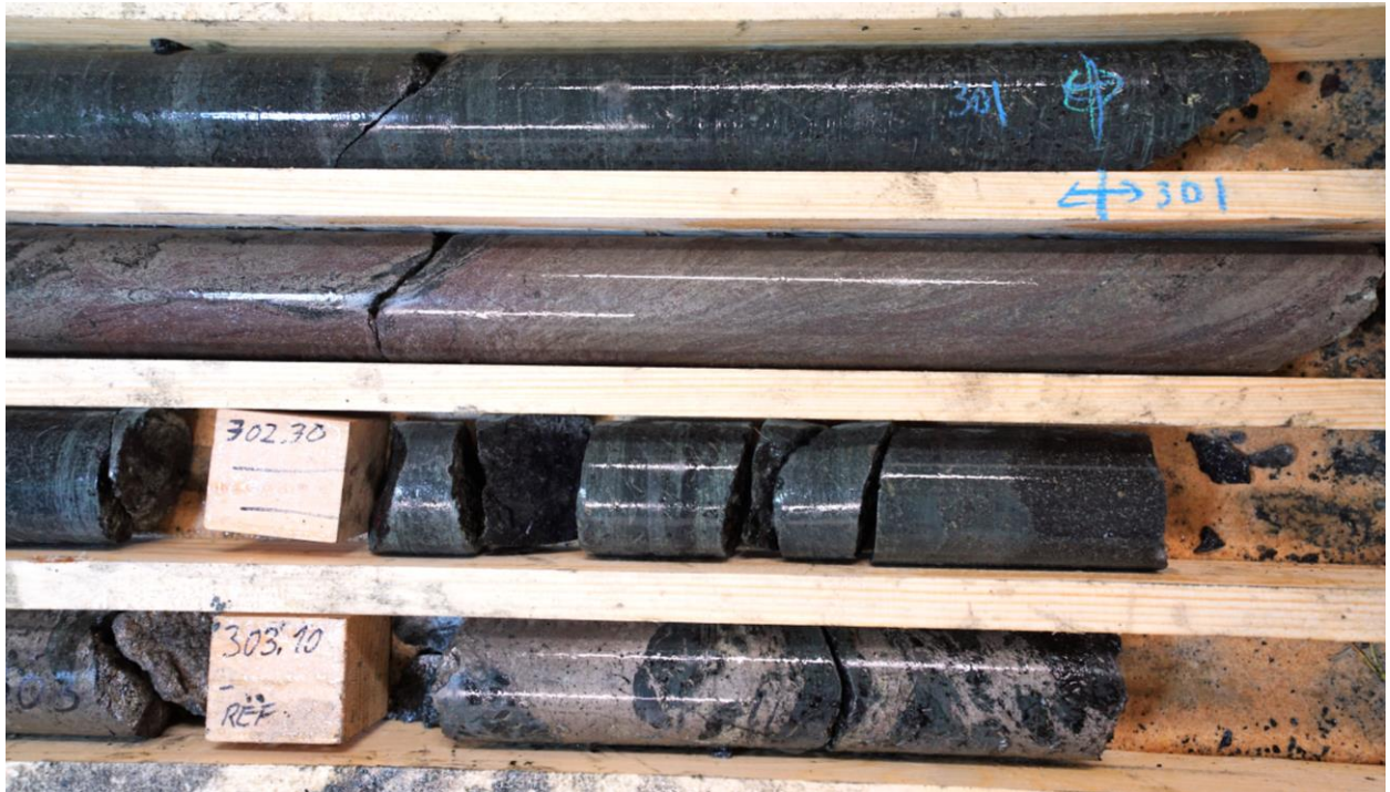
Figure 1. Photograph of massive sulphide zone in hole SBJK170008.
