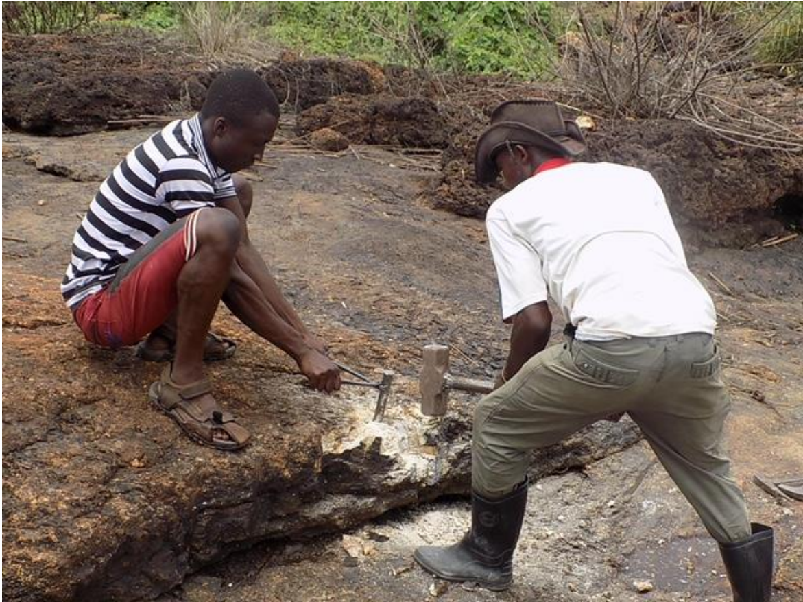
Figure 1: AVZ geologist and field assistant collecting a rock-chip sample of pegmatite from rock exposed in the spillway.
