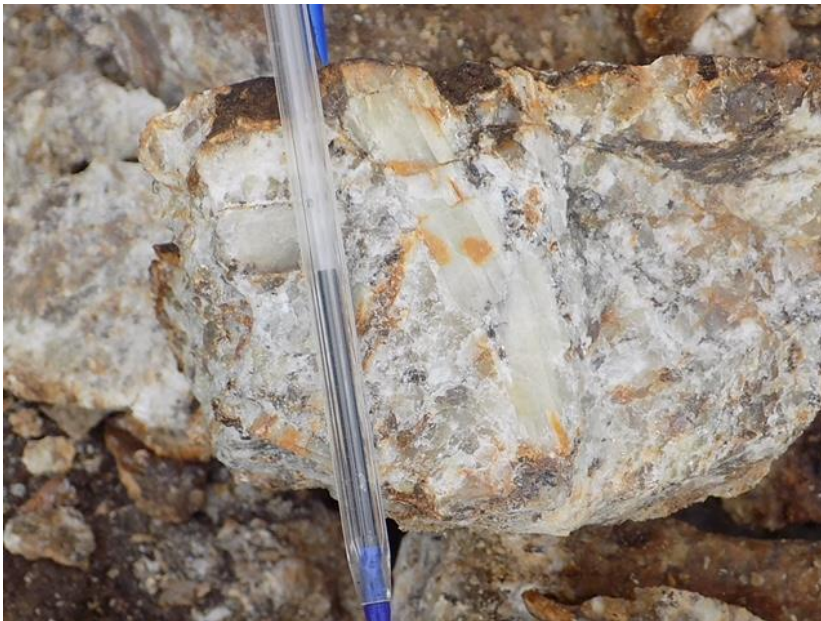
Figure 2: Example of pegmatite sample collected from the spillway outcrops, showing white spodumene (the large, long prism to the right of the blue pen) in a quartz-feldspar matrix.
