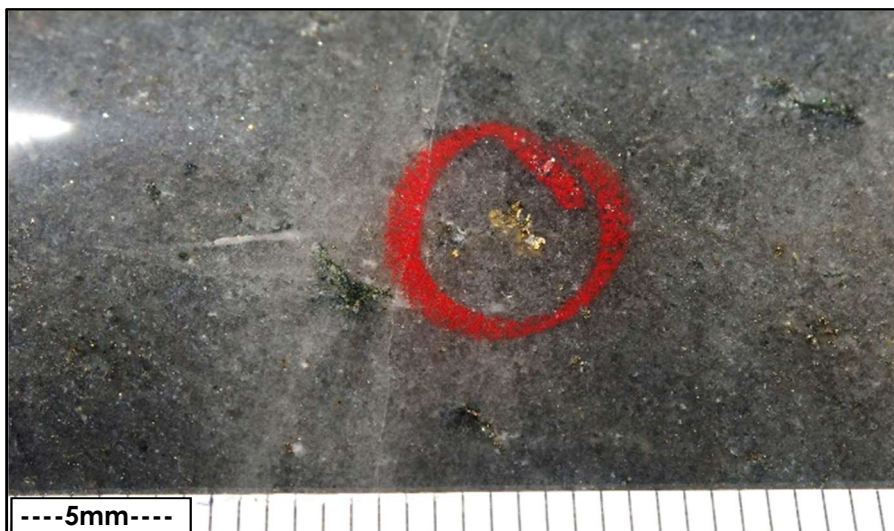
Photo 3: Coarse and Fine grained Visible Gold in New High-grade Lode BBRD0675 132.69m
