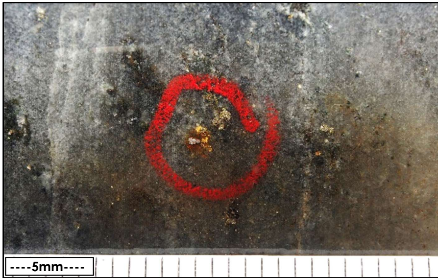
Photo 1: Coarse and Fine grained Visible Gold in New High-grade Lode BBRD0675 132.36m
