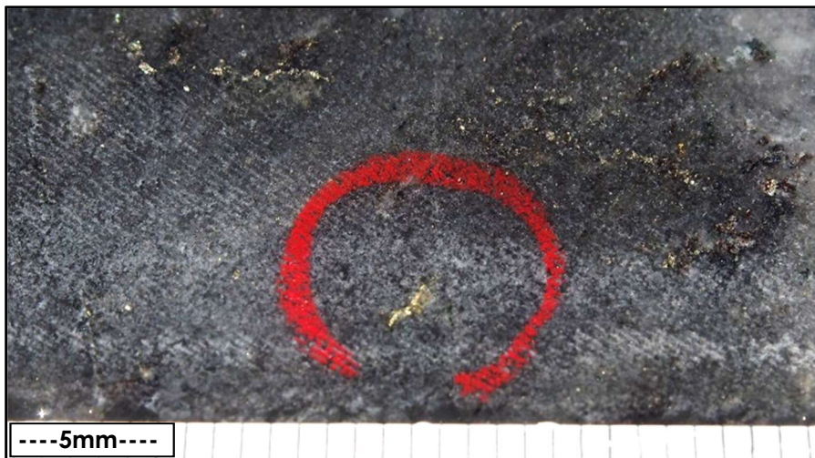
Photo 2: Coarse and Fine grained Visible Gold in New High-grade Lode BBRD0675 132.44m
