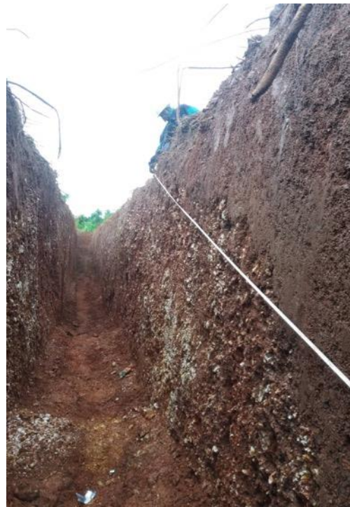
Figures 3 and 4. Trench 008 showing exposed and weathered pegmatite from surface dipping 10° to 15° west and providing upper contact structural data
