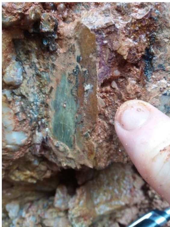
Figures 6 and 7. Partially weathered spodumene lithium mineralisation- exposed in Trench 002 and white spodumene lithium mineralisation from Test Pit 036
