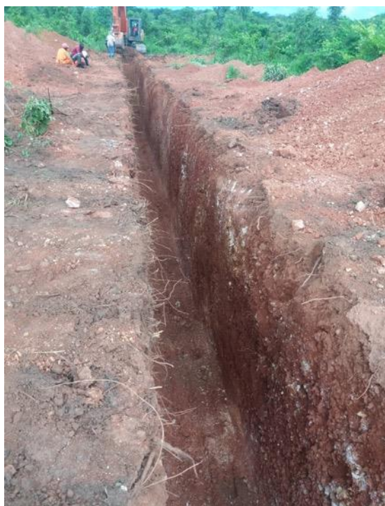
Figures 3 and 4. Trench 008 showing exposed and weathered pegmatite from surface dipping 10° to 15° west and providing upper contact structural data
