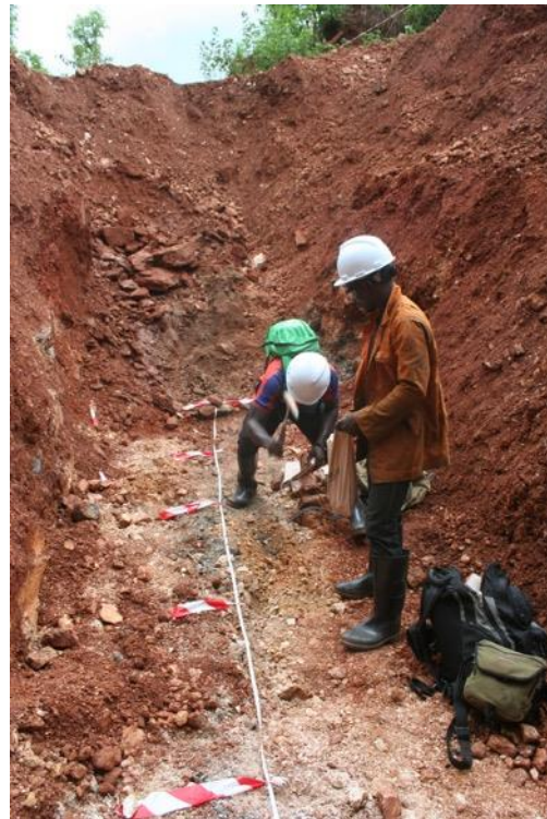
Figures 1 and 2. Commencement of Trench 003 and channel sampling exposed pegmatite at base of Trench 001.
