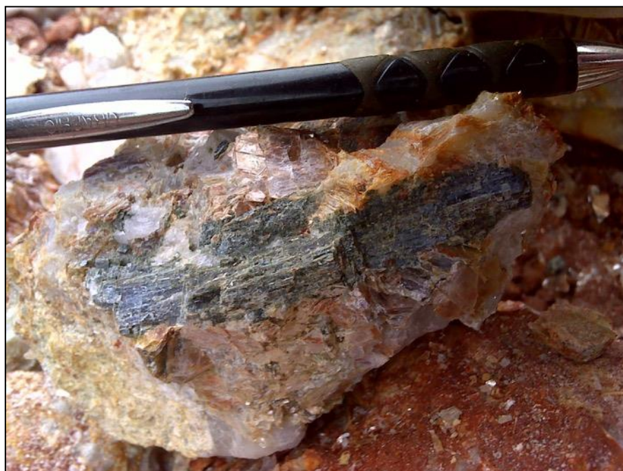
Figure 5. One of several examples of partially weathered spodumene mineralisation – from Trench 008 observed in the trench walls and trench floor.
