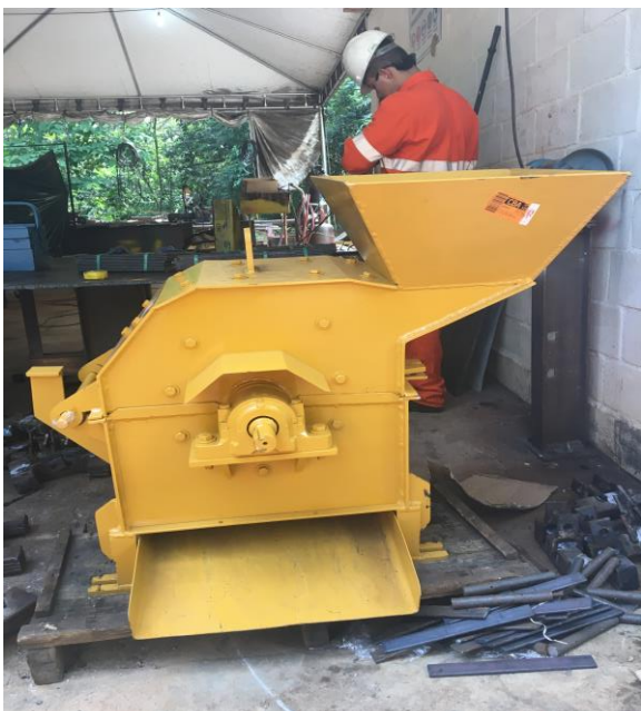
Image 2; 400kg/hr hammer mill
