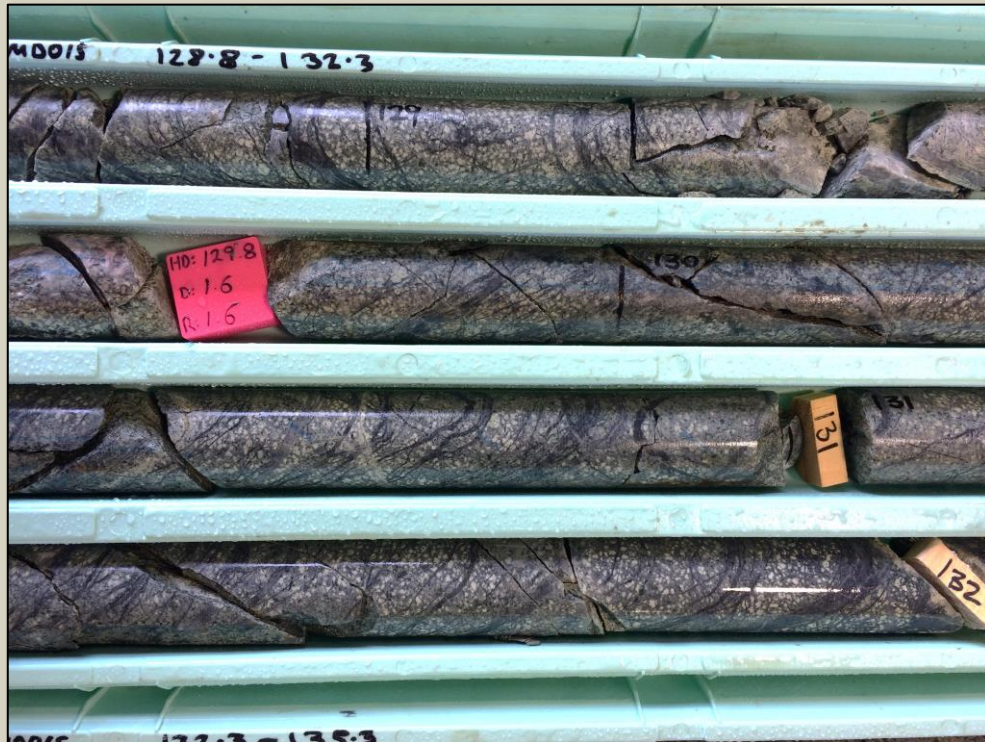
Photo 2. Intense magnetite veining at ~130m in SMD015 from Thursday's Gossan. These veinlets are interpreted to be comparable to Wilson's E-1A veinlets at Cadia Ridgeway.
