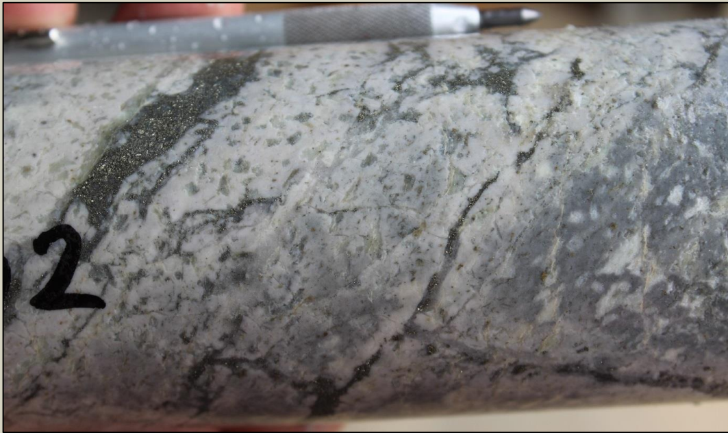
Photo 9. Pyrite-quartz D-veins with sericite alteration halos on the low angle structure at 302 metres in SMD014.
