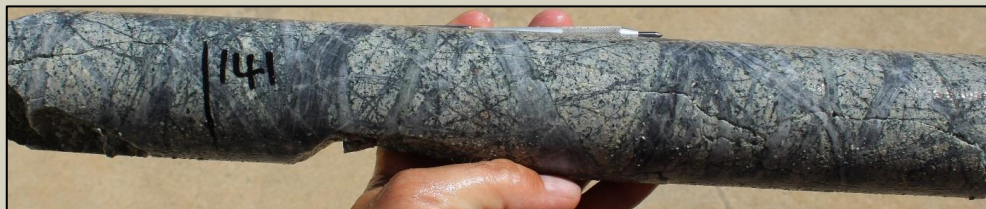
Photo 3. Intense quartz magnetite veining at 141m in SMD015 at Thursday's Gossan. These veins are interpreted to be comparable to Wilson's E-1A and E-1B veinlets described at Cadia Ridgeway.
