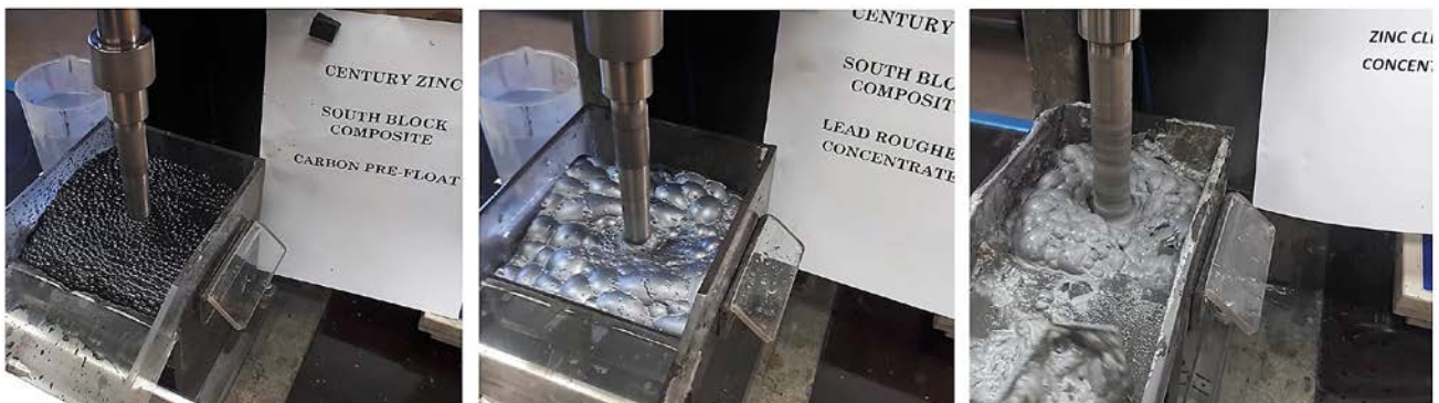
Figure 6: Progressive flotation of the South Block ore samples, with upfront carbon pre-float (left) followed by lead concentrate flotation (middle) and final zinc concentrate flotation (right)
