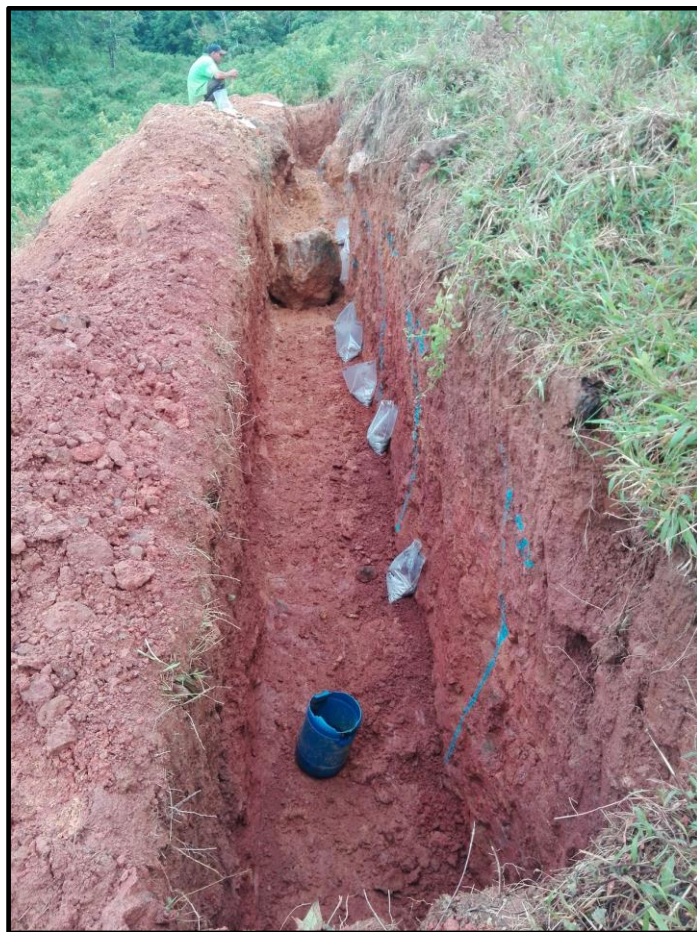
Figure 3 Typical Trench: Sampling of MTNU17034 (Nugget Vein)
