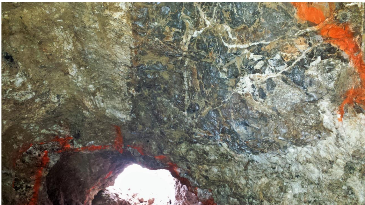
Figure 2 ABOVE: Vein Hv-01 looking back towards the adit of Mine 4494. The wide nature of the vein is evident on the roof of the mine showing the brecciated central part of the vein. Channel samples IM-000481-84 (channel 2) were taken from this approximate location.
