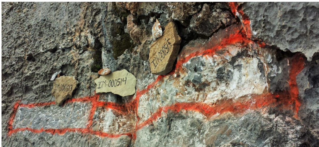
Figure 7 ABOVE : Vein HV-021 sampled with results pending. HV-021 displays very similar traits as HV-01 and HV-02: visible mineralisation, breccia and stockwork fabric.
