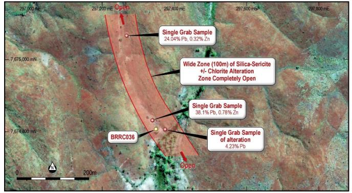
Image 5 – Barker Well Prospect – Location of RC drill-hole BRRC036 and Grab Sample Locations Note: Open in all Directions
