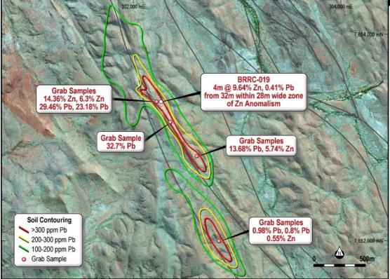
Image 2. Plan of the Devon Cut Prospect Area – RC Drill Hole BRRC019 with Zn in Soil Contouring and Grab Sample Locations. Note: Open in all Directions
