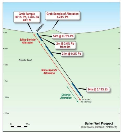
Near the Barker Well Prospect, a single RC drill hole (BRRC036) tested a zone of strona silica sericite alteration approximately 40m south of a small prospect (Barker Well). Previous exploration by Rumble had highlighted a north trending zone with grab sampling returning 38.1% Pb, 24.04% Pb and 4.23% Pb with anomalous Zn. Only three grab samples have been taken in this area (see image 5).
