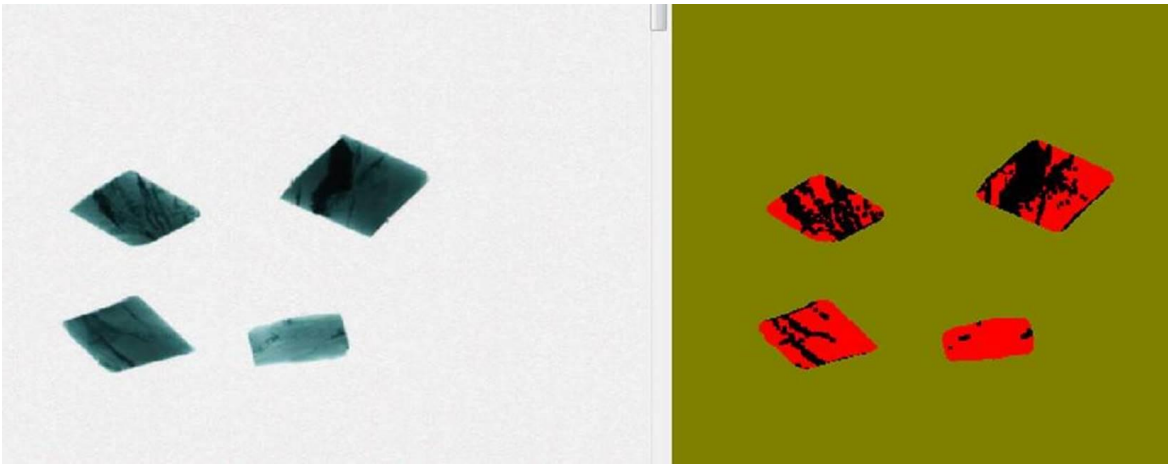
Image 1: Raw XRT image on left shows distinctive cassiterite veining. Classified image on left shows tin as black and host rock as red.
