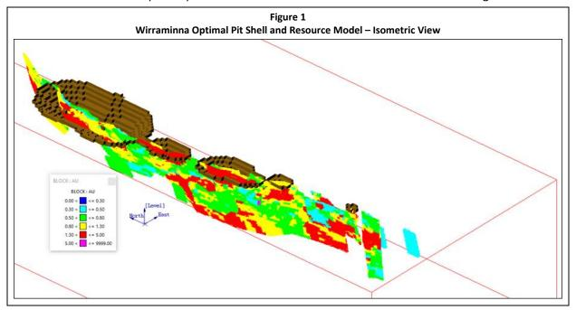
Increasing the overall pit slope to 45 degrees resulted in an approximate 30% increase in contained resource in terms of tonnes and 60% increase in net operating cash flow.
