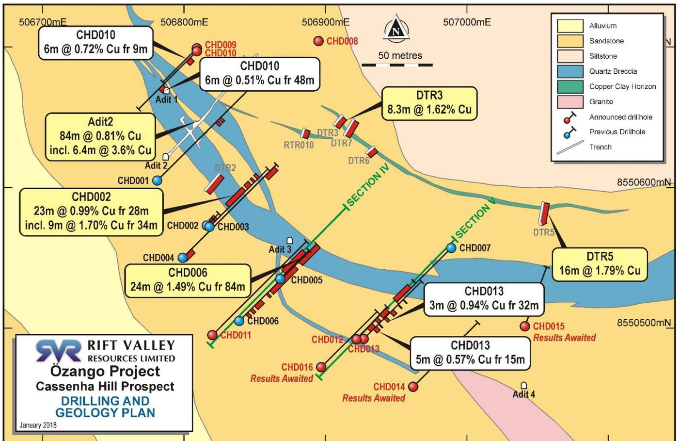
Figure 4: Drill hole location plan of Cassenha Hill with selected intersection highlights from new and previously reported drilling and historic sampling and geology over the 400m strike tested by drilling to date
