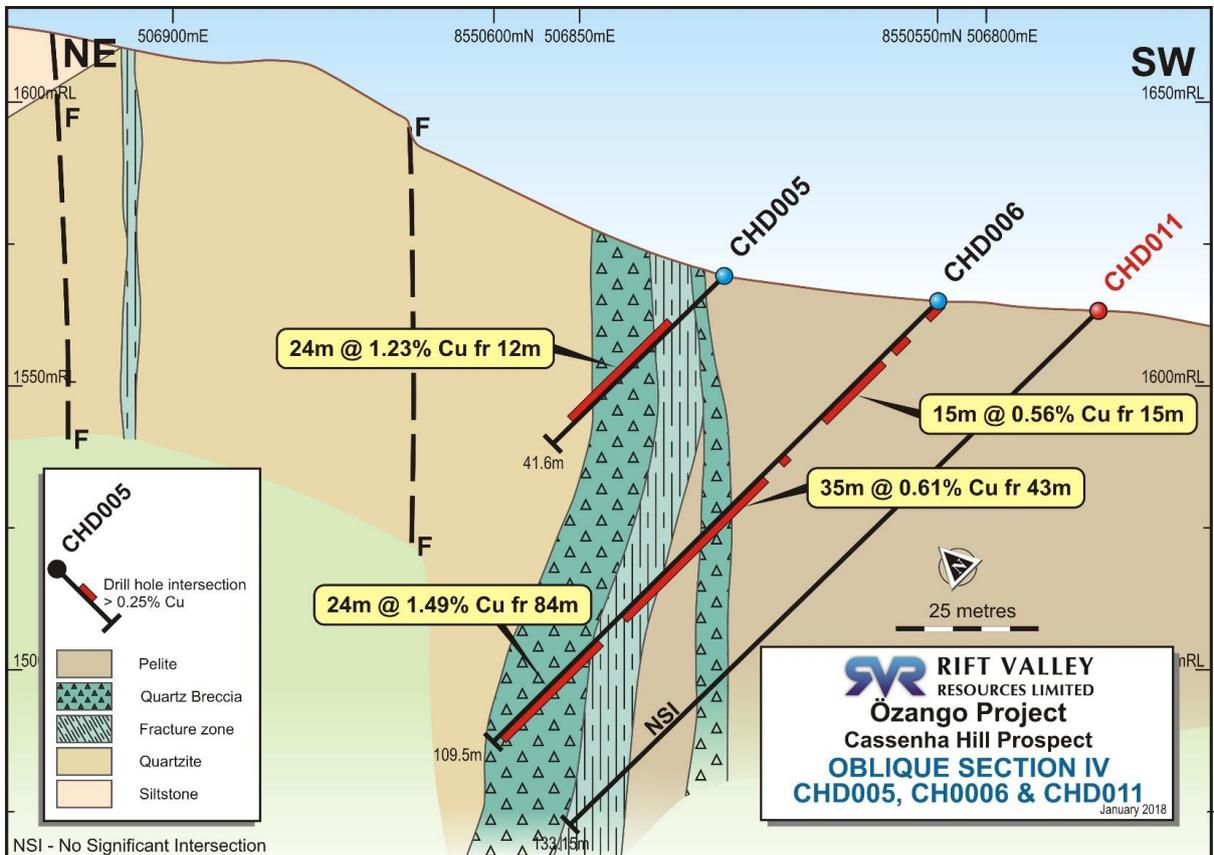
Figure 6: Drill hole cross section of previously reported drilling looking north west showing wide zones of oxide copper mineralisation associated with sub vertical brecciated quartz vein.
