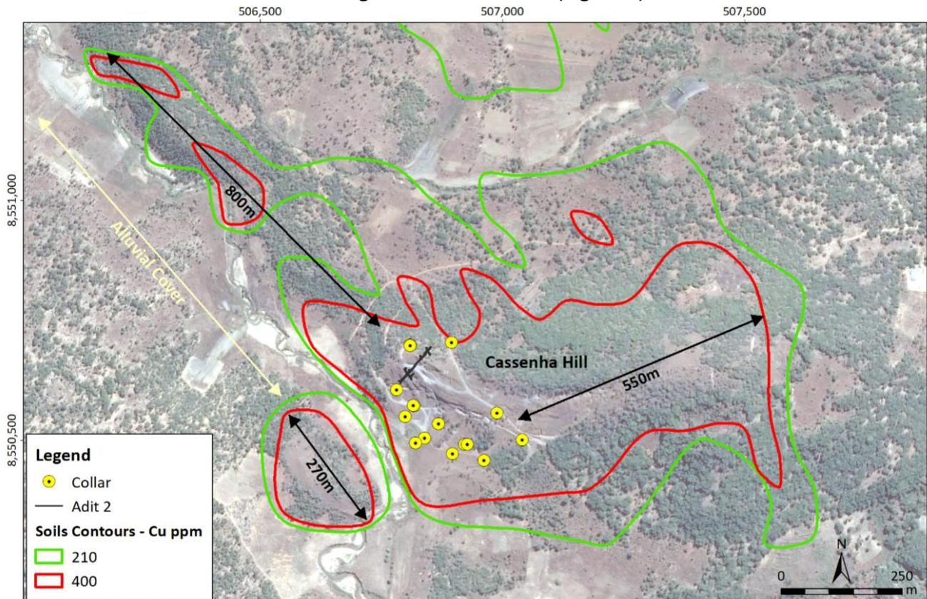
Figure 7: Cassenha Hill drilling over a 400m strike length within the high tenor copper in soil anomaly that extends a further 800m to the north and 550m to the east and currently untested by drilling. Note potential for untested parallel mineralised positions beneath alluvial cover.
