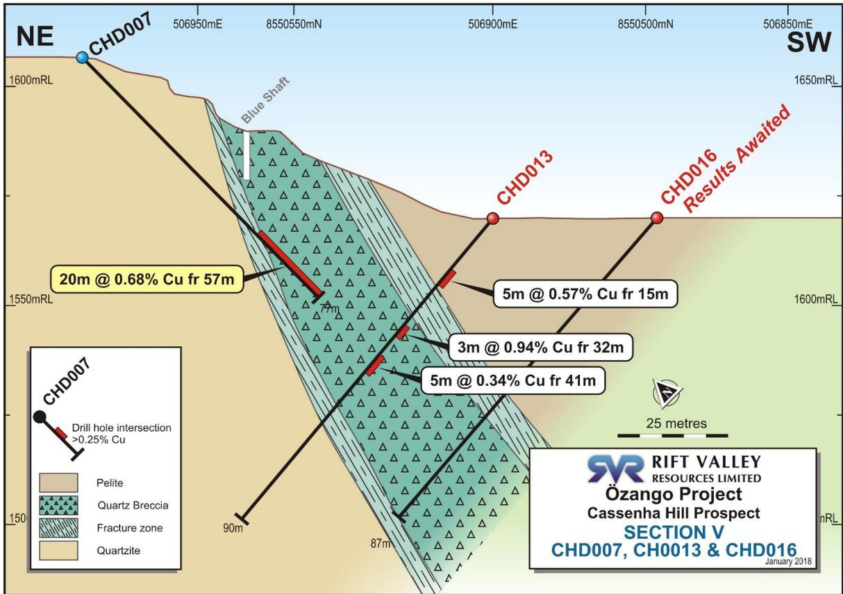
Figure 5: Drill hole cross section of new drilling looking north west (see Figure 4 for location) showing wide zones of oxide copper mineralisation associated with sub vertical brecciated quartz vein.
