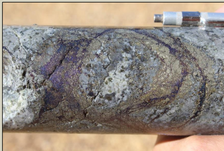
Photo 3. Bornite-chalcopyrite-pyrite ± chalcocite veining at 198.3m in SMD015.
