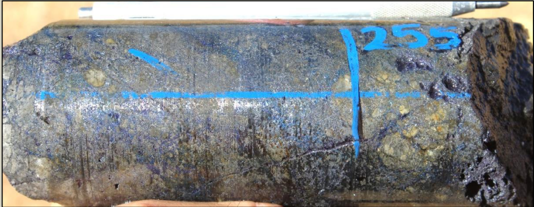
Photo 4. Chalcocite-bornite-pyrite-chalcopyrite veining at 255.0m on the low-angle structure.
