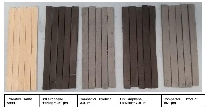
Fig.1 Appearance of coated test specimens
