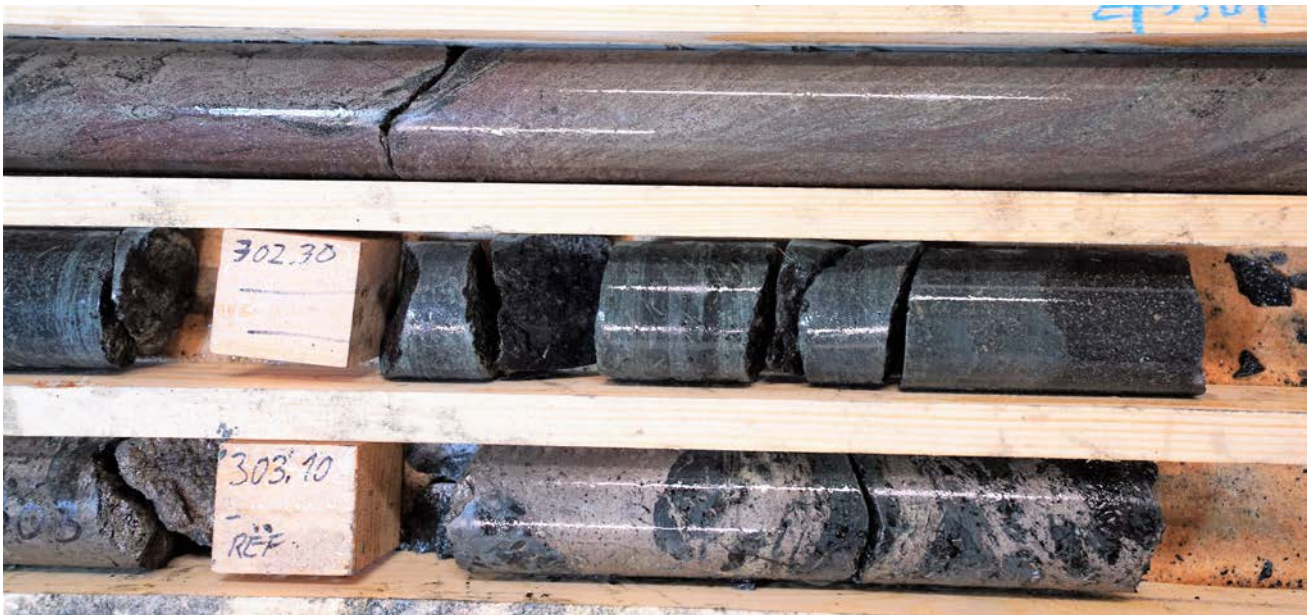
Figure 9. Photo of zinc (sphalerite) rich mineralization in the massive sulphide zone intercepted in hole SBJK17008 at Bjurtraskgruvan.
