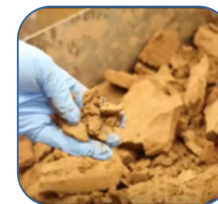
Final flotation concentrate from beneficiation pilot
