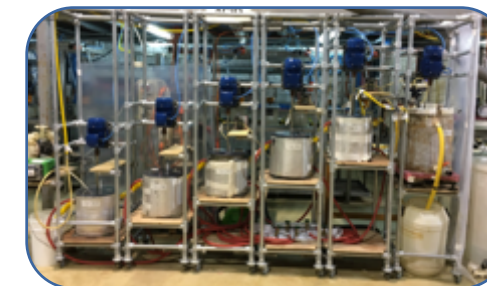
Neutralisation & Precipitation Circuit – Hydromet - ANSTO
