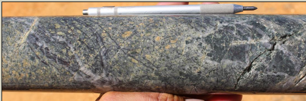
Photo 2. Quartz-magnetite veining at 249m in SMD016.
