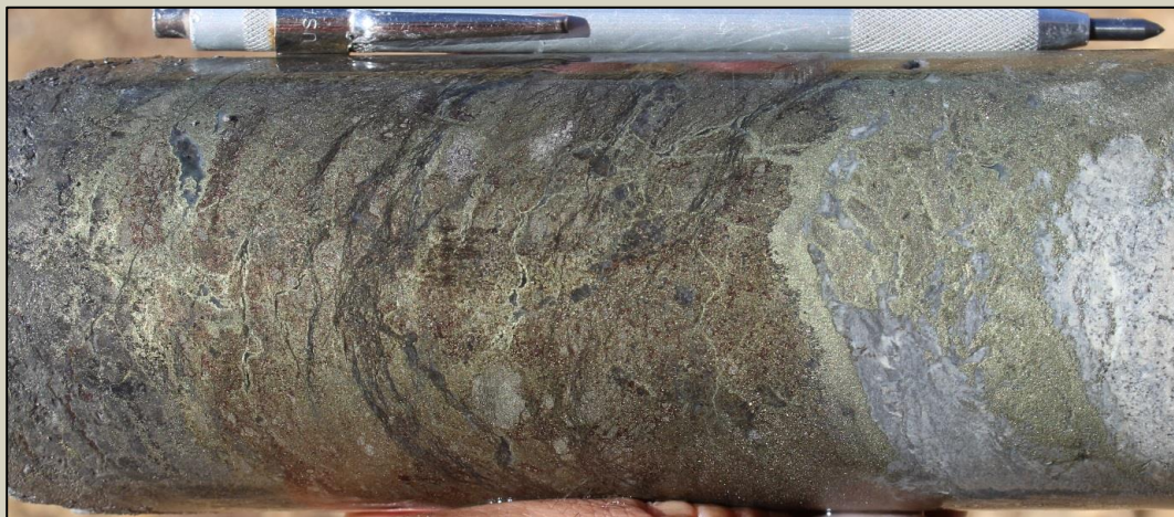
Photo 7. Bornite-chalcopyrite-pyrite 'D' vein beneath the low angle structure at 336.8m.
