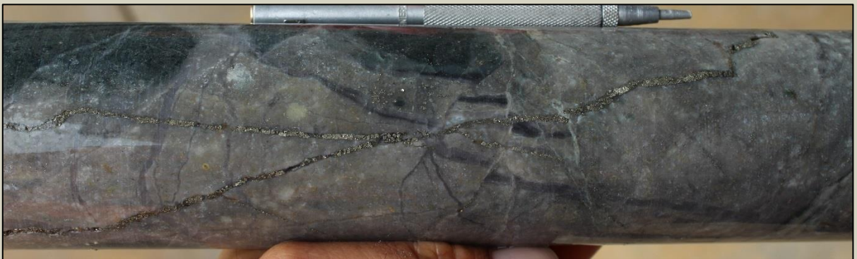
Photo 5. Pyrite vein cutting earlier quartz-sulphide vein at 228.6m.
