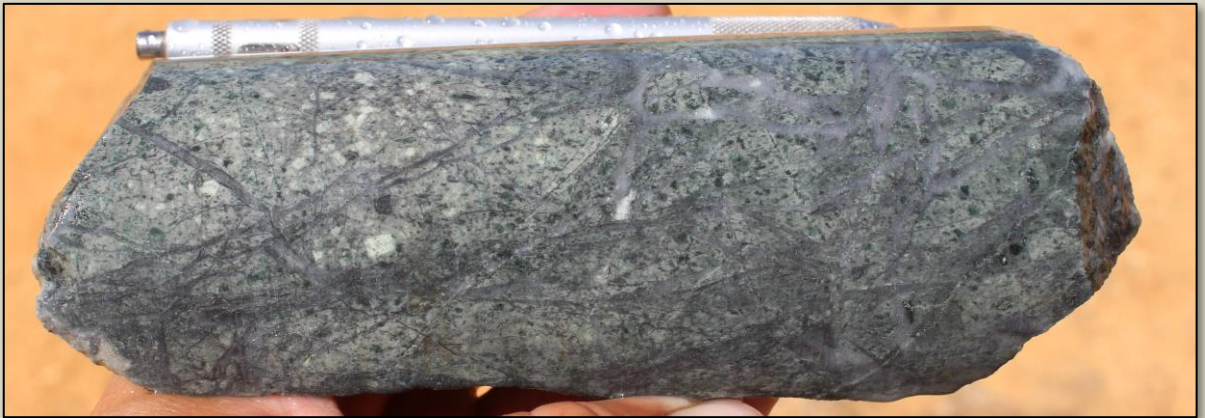
Photo 4. 'M' and 'A' style quartz veins at 256.7m in SMD016.
