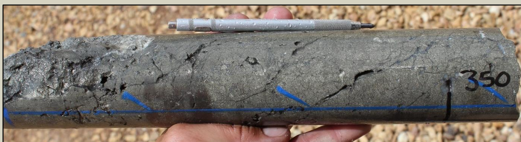
Photo 8. Massive pyrite vein at 350.0m.
