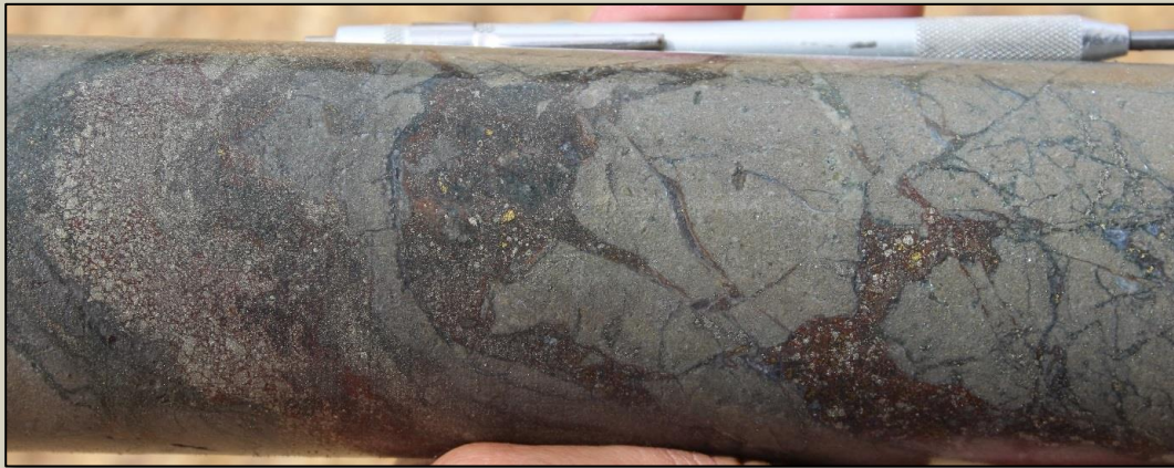
Photo 9. Pyrite-hematite-chalcopryrite-bornite-chalcocite-quartz veining at 364.0m.
