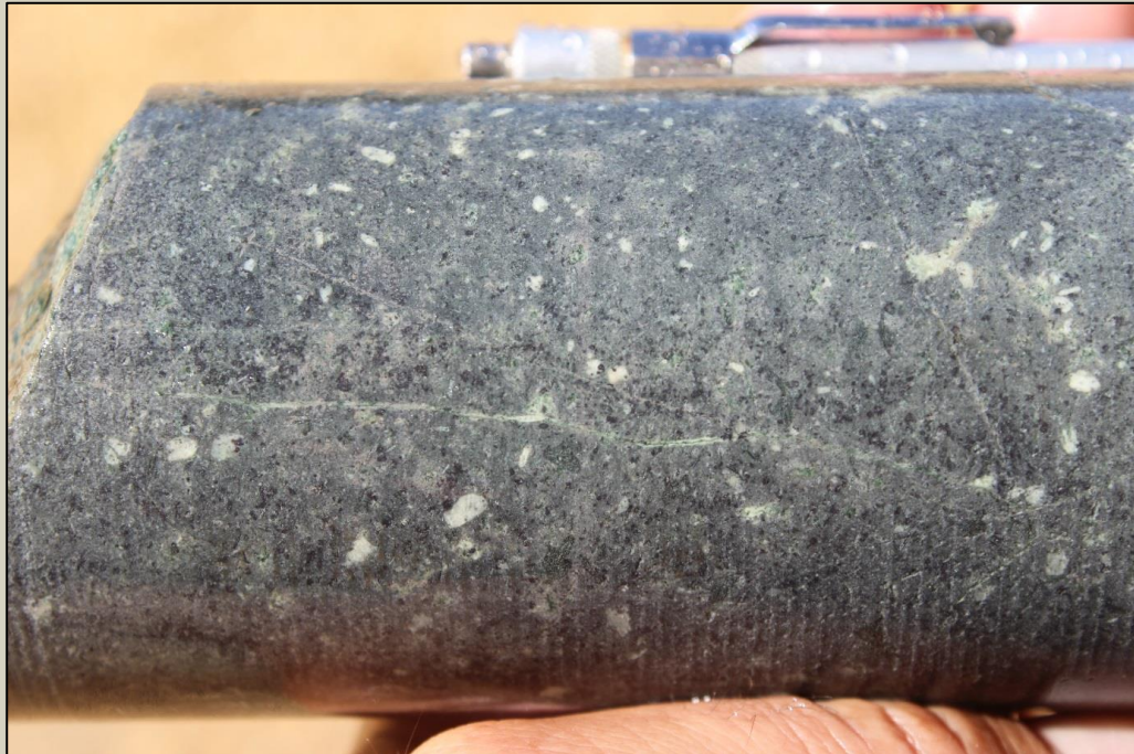
Photo 6. Hematite-magnetite ± actinolite altered porphyritic andesite with very fine trace disseminated bornite and chalcopyrite at 316.2m.
