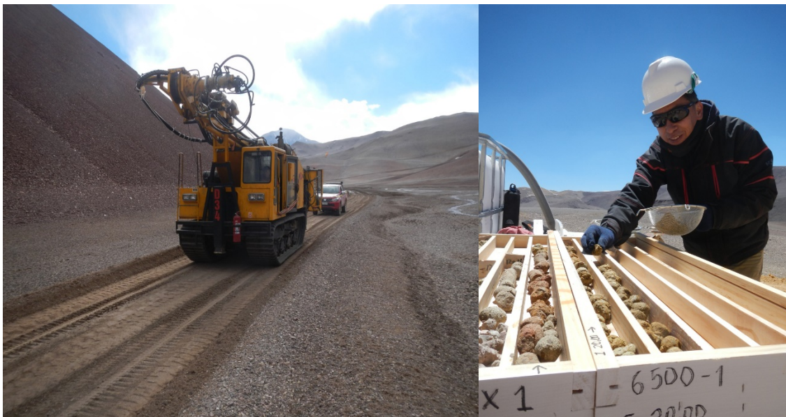
Figure 4: Drilling equipment in transit and air core sample recovery, Vidalita property, Chile
