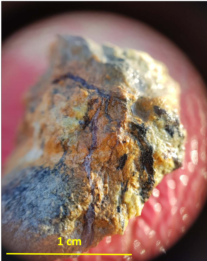
Figure 2: Drill chip from 33.0 to 34.0m interval of air core drill hole 17MDA0100 (28.9 g/t gold and 0.07% copper) with thin iron oxide (possibly ex-sulphide mineralisation) and quartz veining within altered siltstone.
