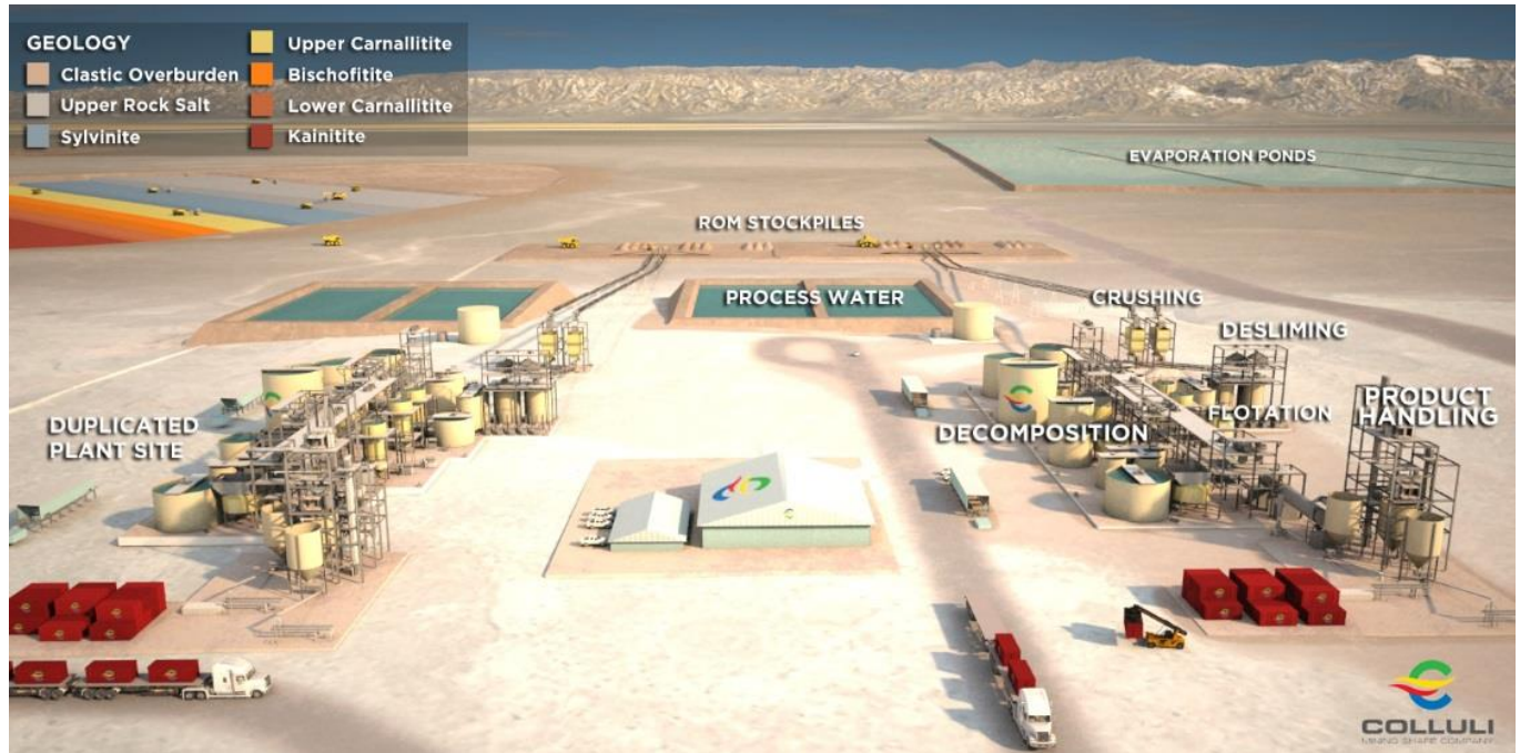
Figure 8: Potential mine layout including key project components for Modules I and II
