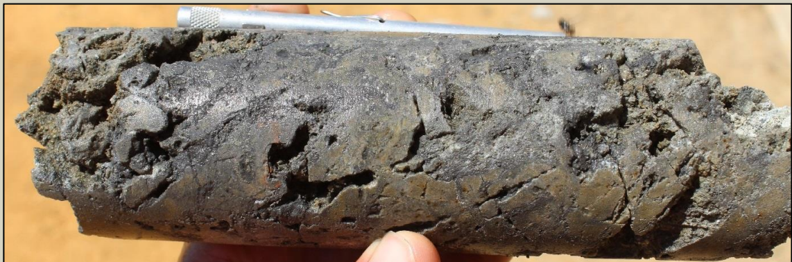
Photo 1. Pyrite-quartz-hematite vein at 183m.
