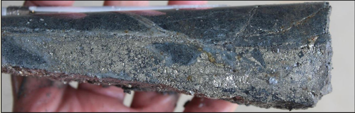
Photo 3. Pyrite-chalcopyrite \pm bornite veining with ?actinolite halo at 322m.
