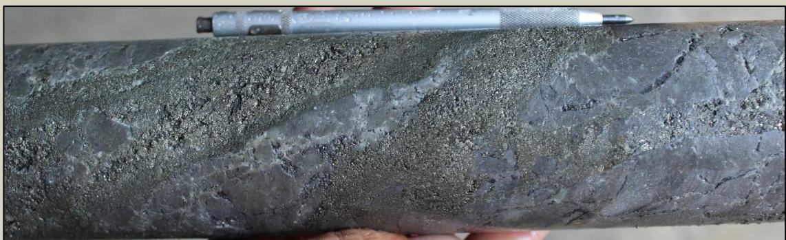
Photo 2. Pyrite-quartz ± sphalerite ± molybdenite veins at 283m.
