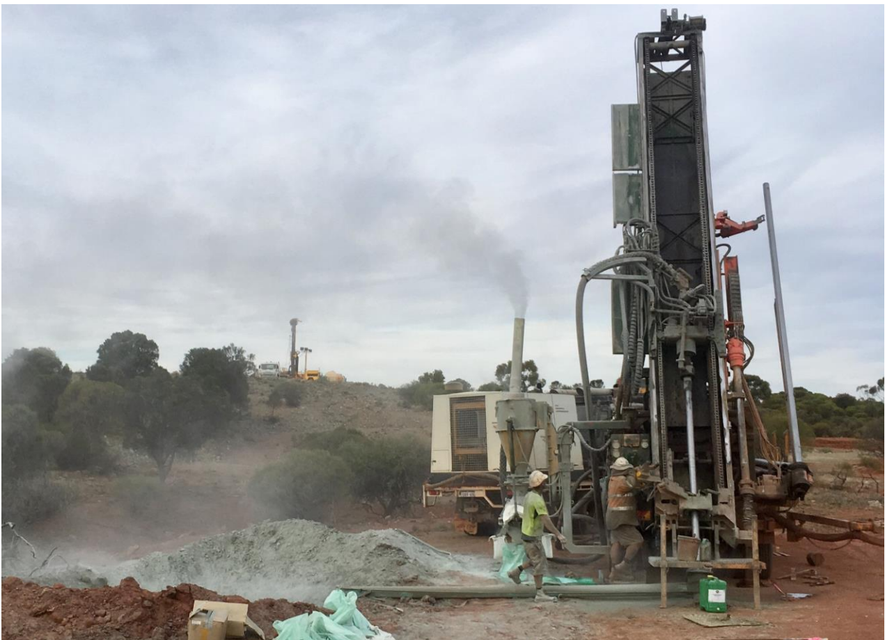
FIGURE 4 – RC RIG DRILLING AT ROTHSAY
