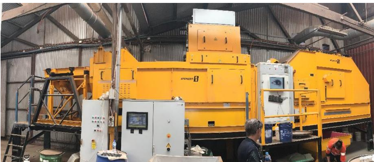
FIGURE 6 – STEINERT MULTI-SENSOR ORE SORTER AT NAGROM IN WESTERN AUSTRALIA
