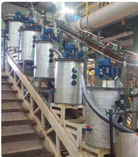
Leach circuit at SGS Metallurgy pilot plant
