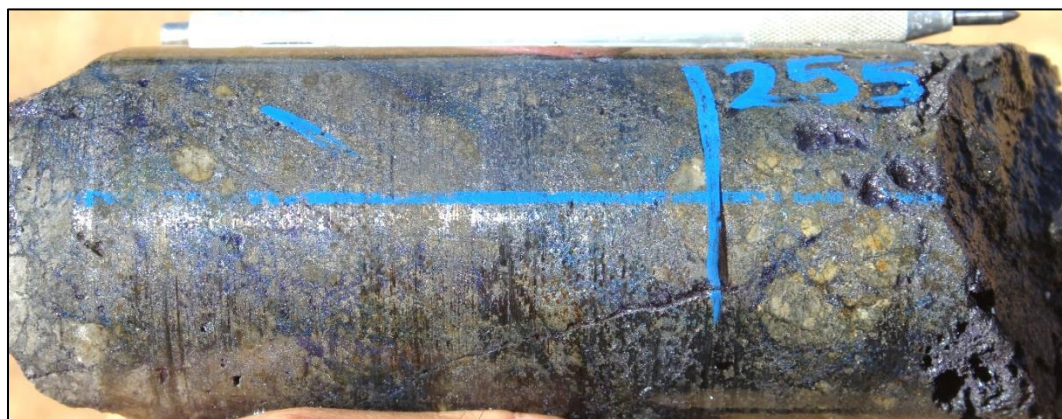
Photo 10. Chalcocite-bornite-pyrite-chalcopyrite veining at 255.0m on the low-angle structure.
