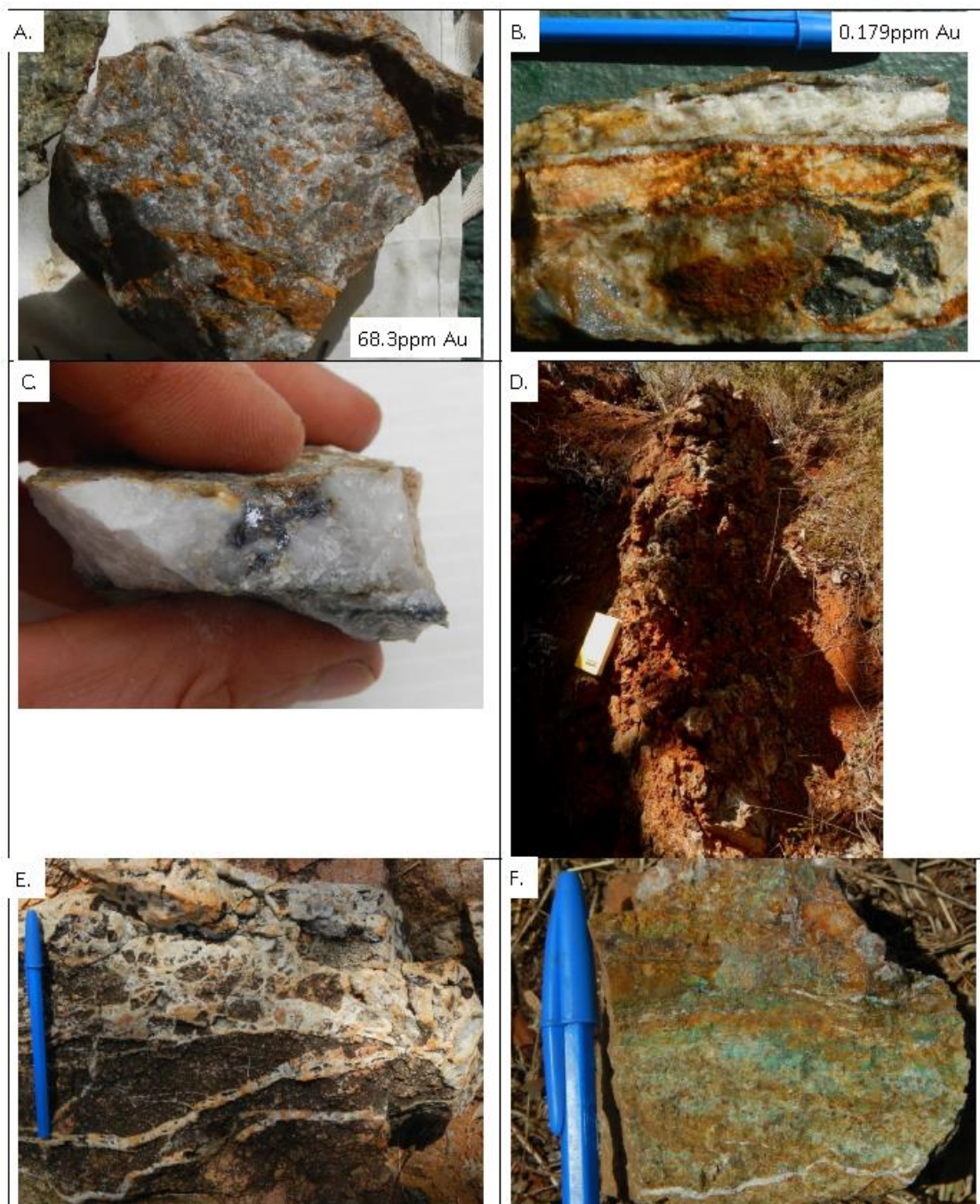
Photo 11. A. Quartz+carbonate+siderite breccia vein from Albion North, trending 357° B. Multi-generation quartz+calcite+siderite breccia vein from the Highway mine C. Quartz+galena vein. Albion workings D. Calcite+quartz vein trending 69/255°, from the Ellen Boss workings E. Stockwork quartz veins in granite and quartz-cemented granite-clast breccia from east of Rejoice. F. Sheeted quartz+calcite veins with abundant secondary copper carbonate, Percy Keene Junior workings.
