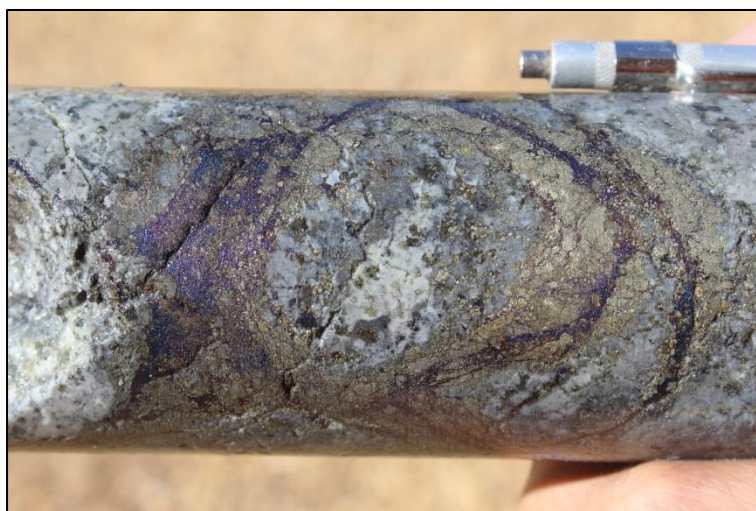
Photo 9. Pyrite-bornite-chalcopyrite-chalcocite veining at 198.3m in SMD015.
