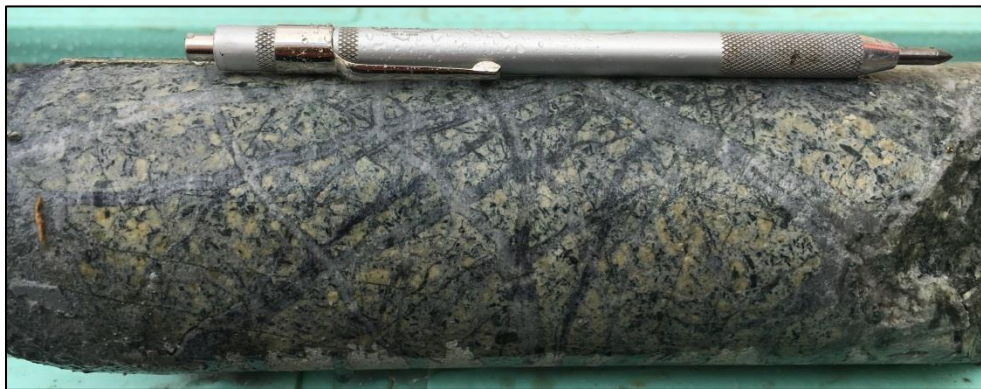
Photo 7. Magnetite and quartz-magnetite veining at 154.0m in SMD015.
