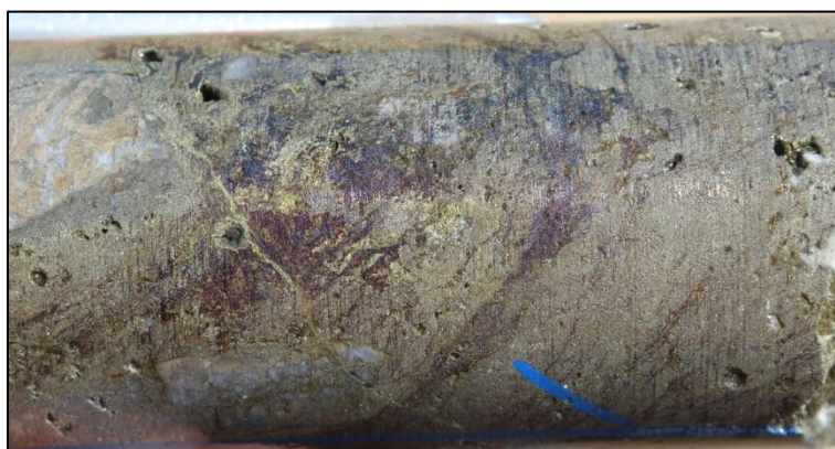
Photo 8. Pyrite-bornite-chalcopyrite ± chalcocite vein at 196.6m in SMD015. Bornite is the purple sulphide. Drill core is HQ3 with a diameter of 61mm.
