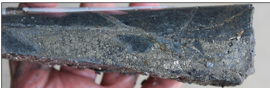
Photo 2. Pyrite-chalcopryite \pm bornite veining with ?actinolite halo at 322m.
