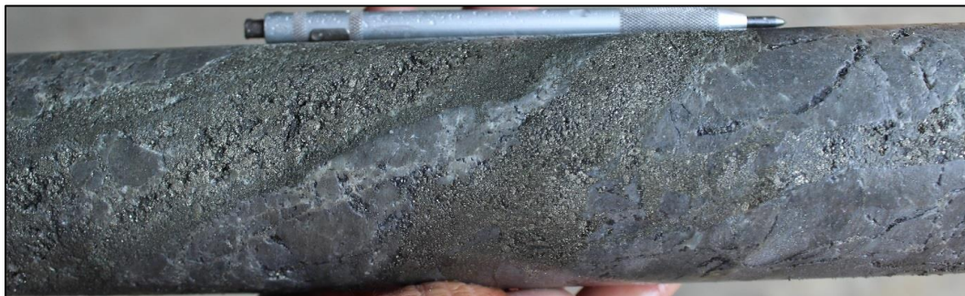
Photo 1. Pyrite-quartz \pm sphalerite \pm molybdenite veins at 283m.
