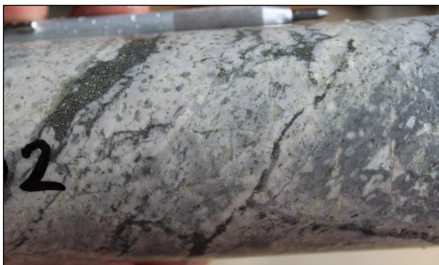
Photo 6. Pyrite-quartz 'D' veins with sericite alteration halos on the low angle structure at 302 metres in SMD014.
