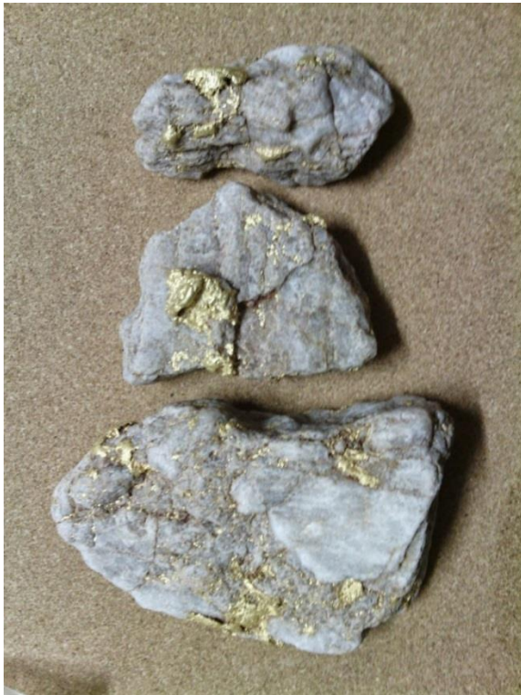
Figure 18. High Grade Gold in Quartz from P53/1627 (largest specimen approximately 10cm in length)
