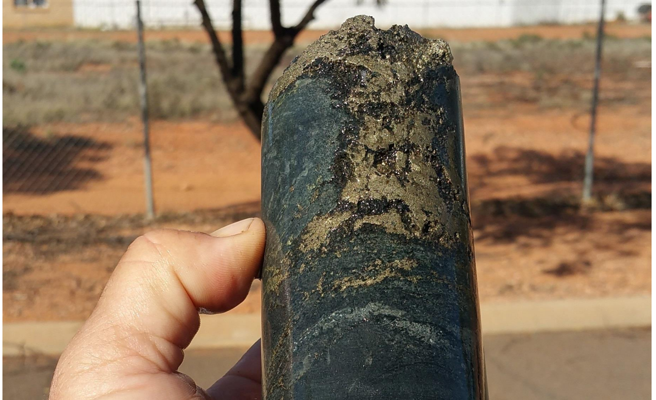
Figure 2. Photograph of a bleb of semi massive nickel sulphide at approximately 125.4m downhole in NCB0001. This sulphide is interpreted to be remobilised into the pillow margins of the footwall basalt sequence from the CBLC.
