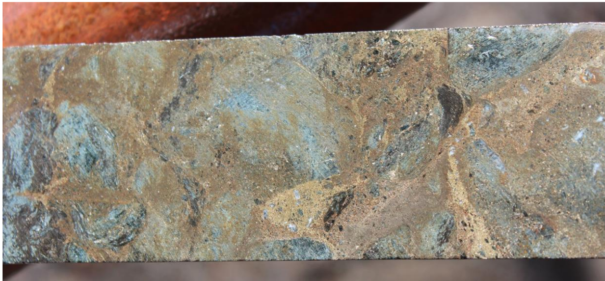
Figure 12. Nickel sulphides in drill core from Spargoville.
