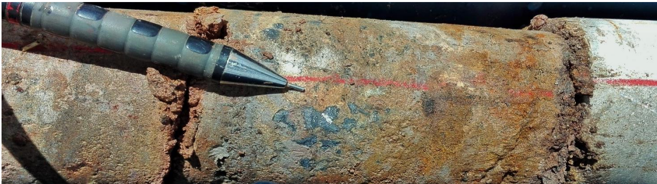
Figure 2 BELOW : Core photo of manto horizon at 42.1m in RDDH-022. The manto grades 20.77% Zn, 95.7g/t Ag and 6.73% Pb over 0.3m.
