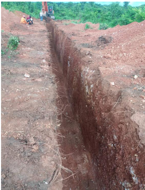
Figures 14 and 15: Trench 008 showing exposed and weathered pegmatite from surface dipping 10^{\circ} to 15^{\circ} west and providing upper contact structural data
