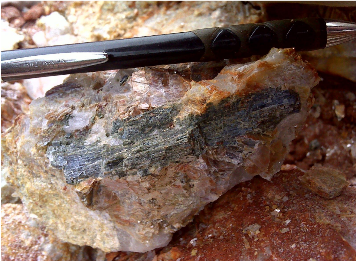
Figure 16: One of several examples of partially weathered spodumene lithium mineralisation – from Trench 008 observed in the trench walls and base.
