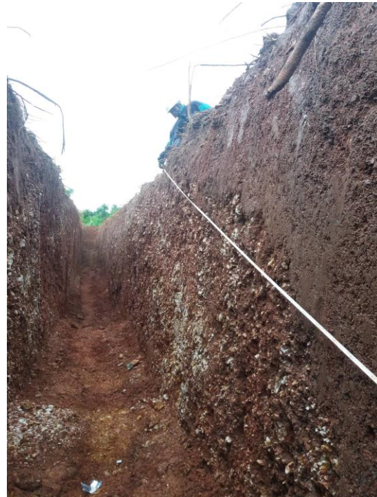
Figures 14 and 15: Trench 008 showing exposed and weathered pegmatite from surface dipping 10^{\circ} to 15^{\circ} west and providing upper contact structural data
