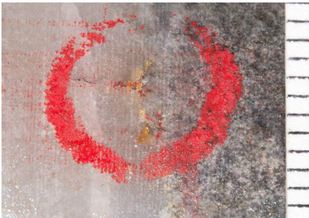
Figure 7. Free gold at 264.70m in TGGRCDD110 (scale: mms).
