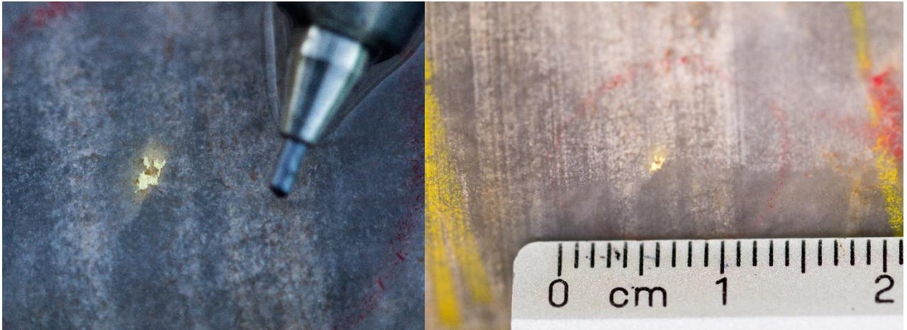
Figure 2. Visible free gold observed in drill core at 128.80m down hole TGGDD090 at Crown Prince.
