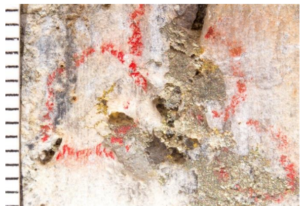
Figure 6. Free gold and sulphide at 264.10m in TGGRCDD110 (scale: mms).
