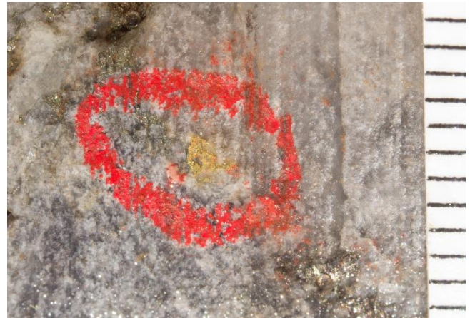
Figure 8. Free gold and sulphide at 264.80m in TGGRCDD110 (scale: mms).
