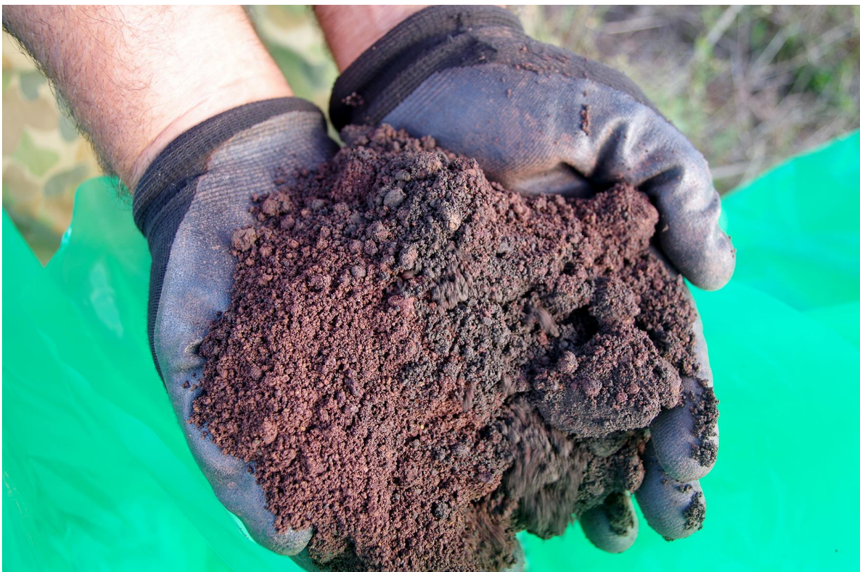
Figure 1: The cobalt-nickel-scandium ore body at Australian Mines' 100%-owned Sconi project is highly friable, making mining and crushing / processing relatively simple.
