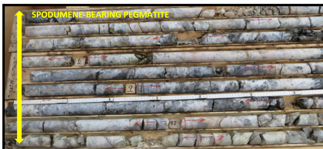
Figure 18. Drill core obtained from drill hole SA-17-15 showing the intersection of a portion of high-quality spodumene-bearing pegmatite from 2m down hole (the lighter coloured material in the photo is the Pegmatite, whilst the darker material is Mafic Volcanic).
