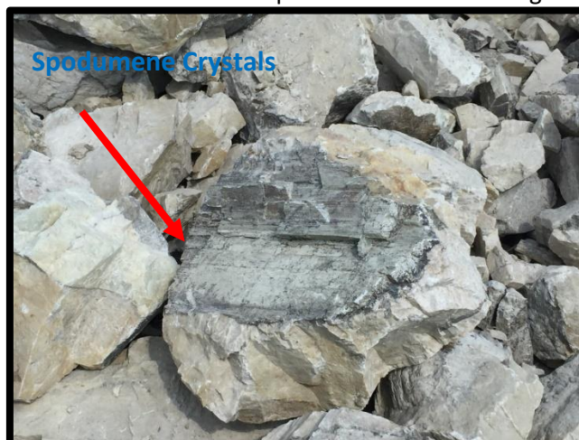
Figure 8. Bulk sample of Spodumene bearing pegmatite obtained from the North Aubry prospect.
