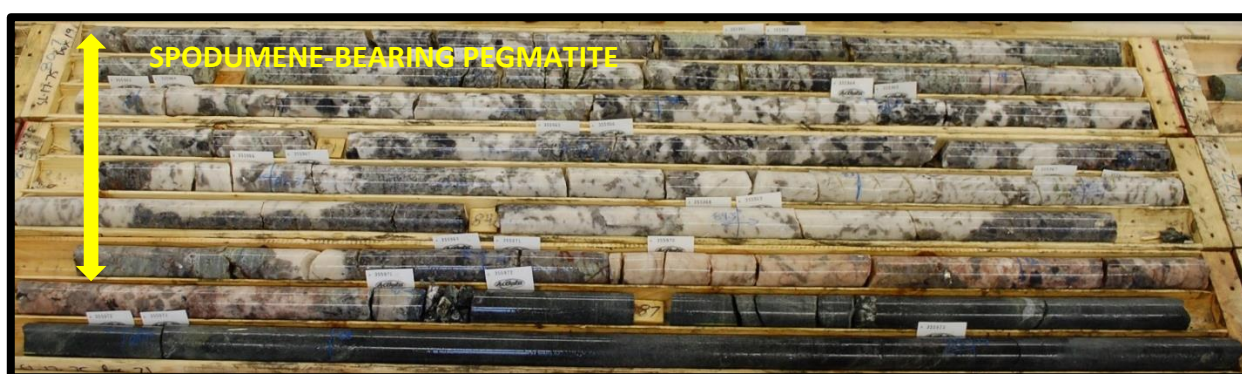
Figure 16. Drill core obtained from drill hole SL-17-75 (from 76.4.8m to 89.0m) showing the intersection of high-quality spodumene-bearing pegmatite (the lighter coloured material in the photo is the Pegmatite, whilst the darker material is Mafic Volcanic).
