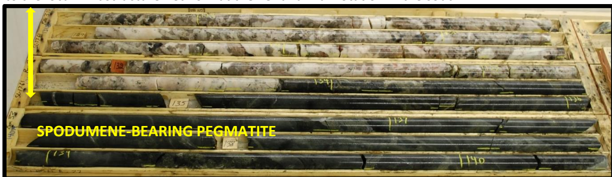
Figure 15. Drill core obtained from drill hole SL-17-61 (core from 127.6m to 140.4m) showing the intersection of high-quality spodumene-bearing pegmatite (the lighter coloured material in the photo is the Pegmatite, whilst the darker material is Mafic Volcanic).
