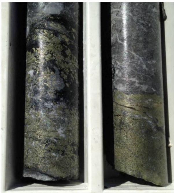
Drill core CCD03 — semi-massive chalcopyrite bands.
