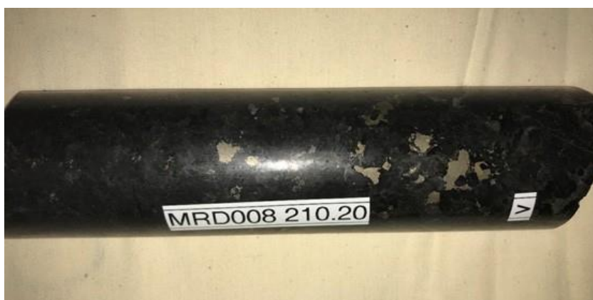
Figure 2. Blebby sulphides hosted in coarse grained pyroxene-olivine mesocumulate showing visible pentinite and chalcocopyrite.
