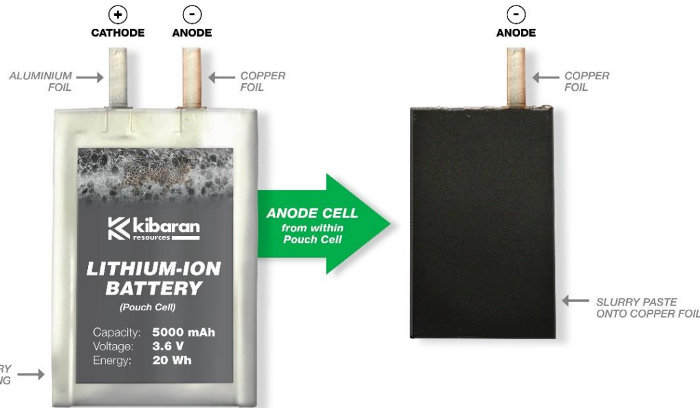
Section through the anode cell showing Epanko Battery (Spherical) Graphite coated on to the anode copper foil
